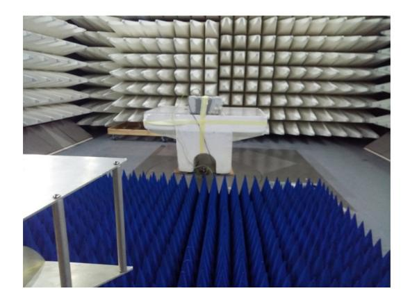
$\label{eq:Photograph No.6} Photograph No.6 \\ Spurious emissions measurement setup at the OATS in 18 – 27 GHz$
