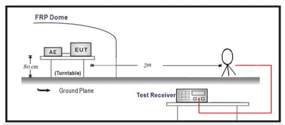
Below 1GHz Test Setup:
