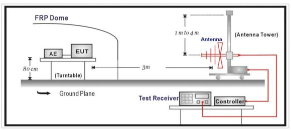
Above 1GHz Test Setup:
