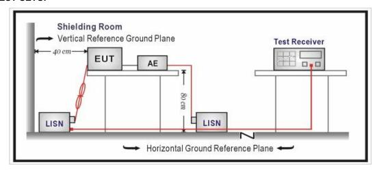
NOTE: For the actual test configuration, please refer to the attached file (Test Setup Photo).
