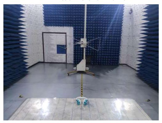
RADIATED EMISSION TEST SETUP ABOVE 1GHz
