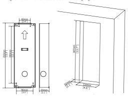
(2) Keep the recess bracket facing outward and upward, and insert four pointed tail cross screws into inside holes to secure the bracket on the wall.
