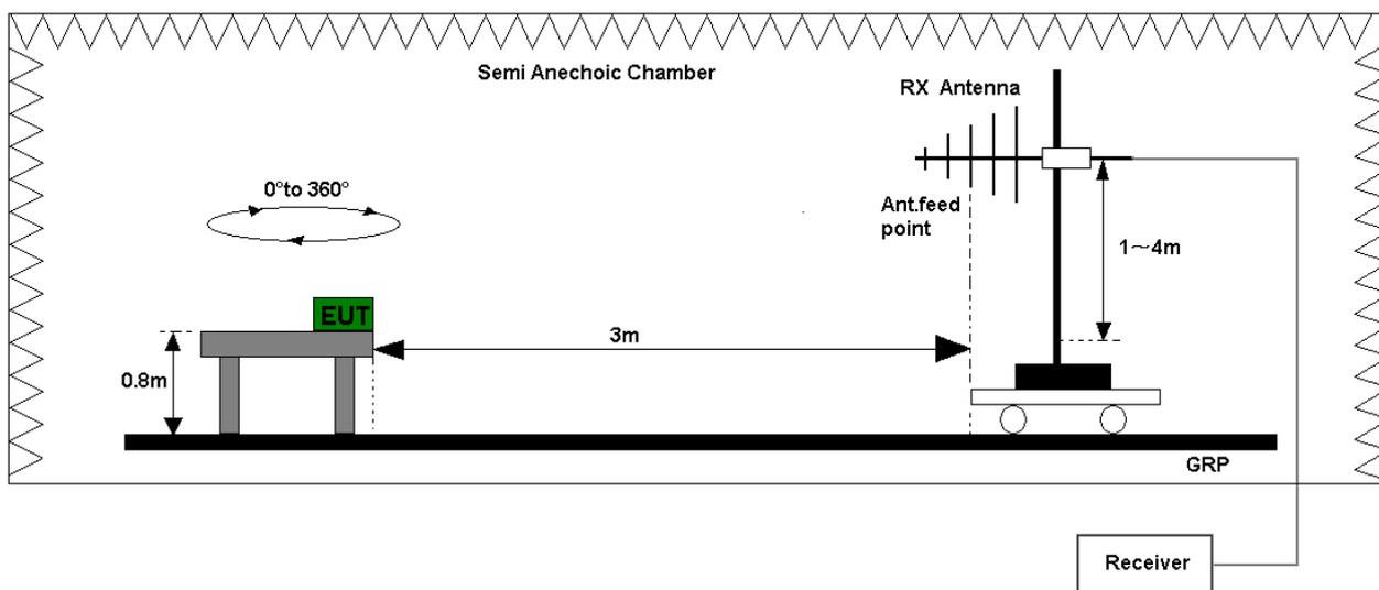
Figure 1. Test set-up of radiated disturbance(30MHz-1GHz )
