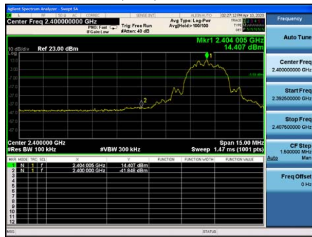
BT UHD 2M 8DPSK, Carrier frequency (MHz): 2404
