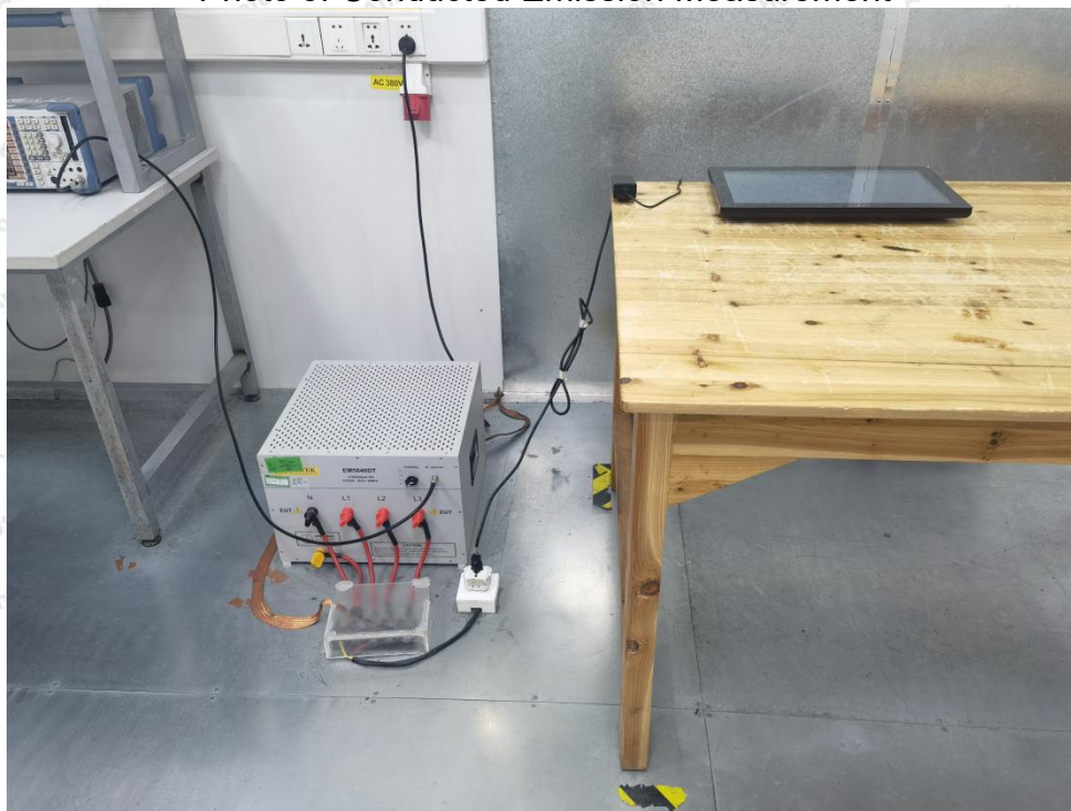
Photo of Conducted Emission Measurement
