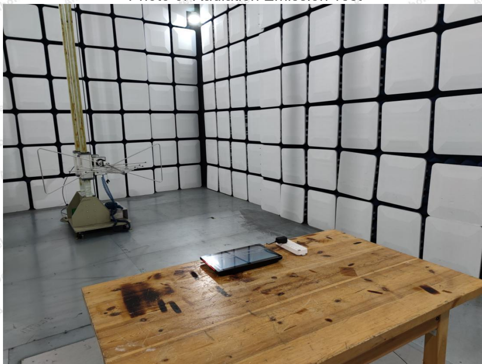
Photo of Radiation Emission Test
