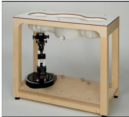
Picture C.10: SAM Twin Phantom
