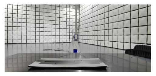
Radiated emission test: Frequency Range< 30MHz ~1GHz >
