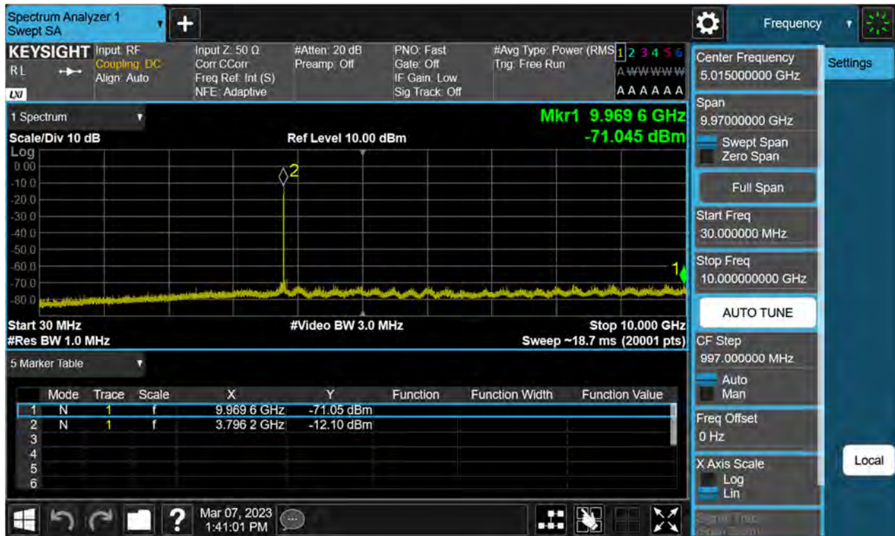
Sub6 n77(78). Conducted Spurious Plot_1 (656000ch_90 MHz_BPSK)
