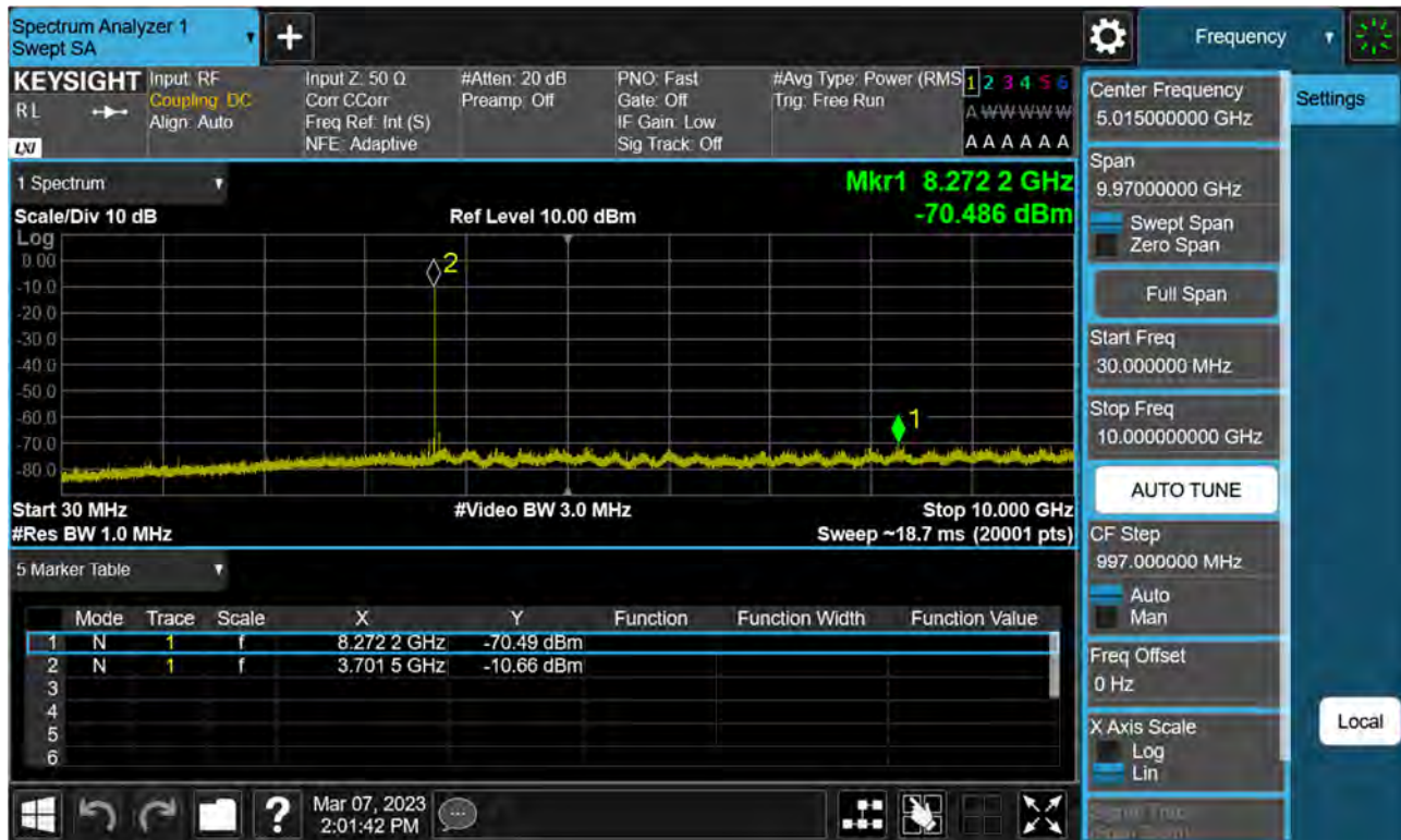
Sub6 n77(78). Conducted Spurious Plot_1 (650000ch_100 MHz_BPSK)
