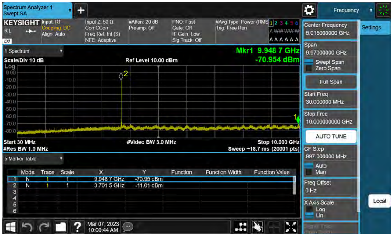
Sub6 n77(78). Conducted Spurious Plot_1 (647334ch_20 MHz_BPSK)
