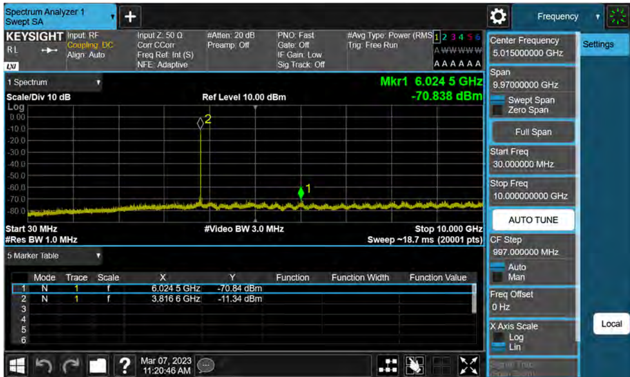
Sub6 n77(78). Conducted Spurious Plot_1 (656000ch_50 MHz_BPSK)
