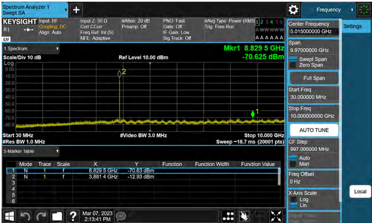
Sub6 n77(78). Conducted Spurious Plot_1 (662000ch_100 MHz_BPSK)
