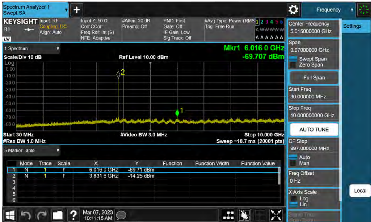
Sub6 n77(78). Conducted Spurious Plot_1 (656000ch_20 MHz_BPSK)
