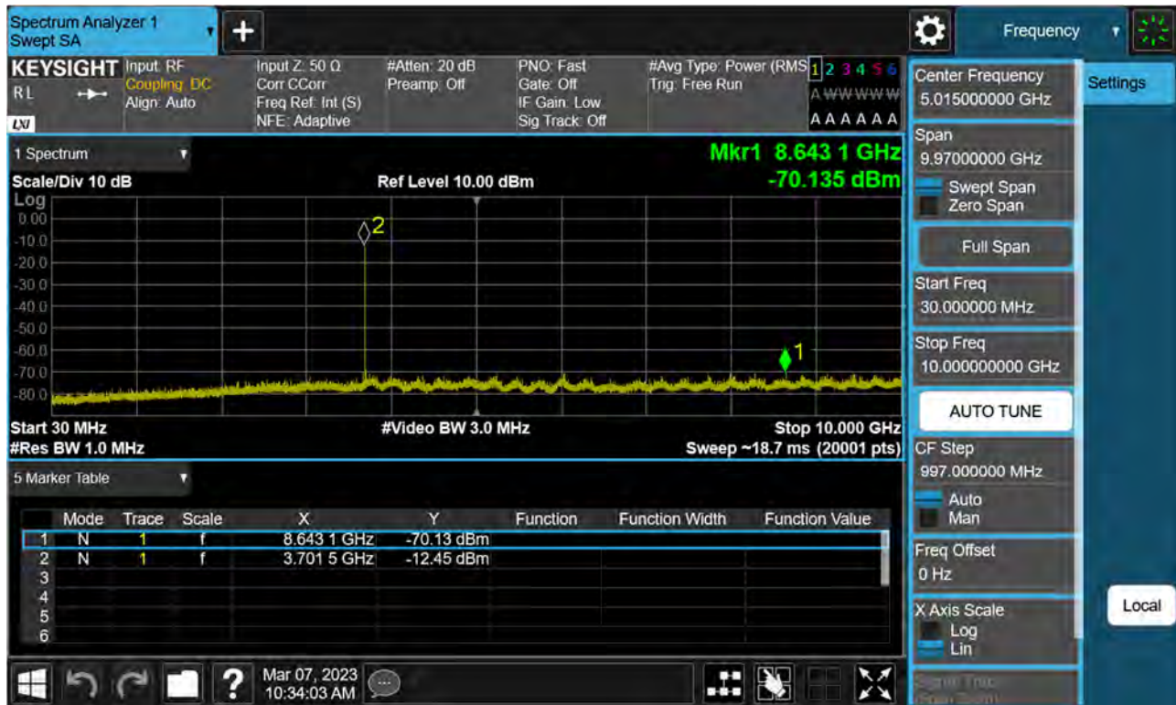
Sub6 n77(78). Conducted Spurious Plot_1 (648000ch_40 MHz_BPSK)
