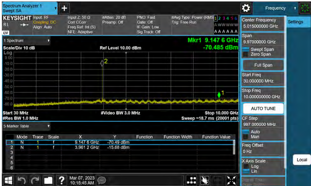
Sub6 n77(78). Conducted Spurious Plot_1 (664666ch_20 MHz_BPSK)
