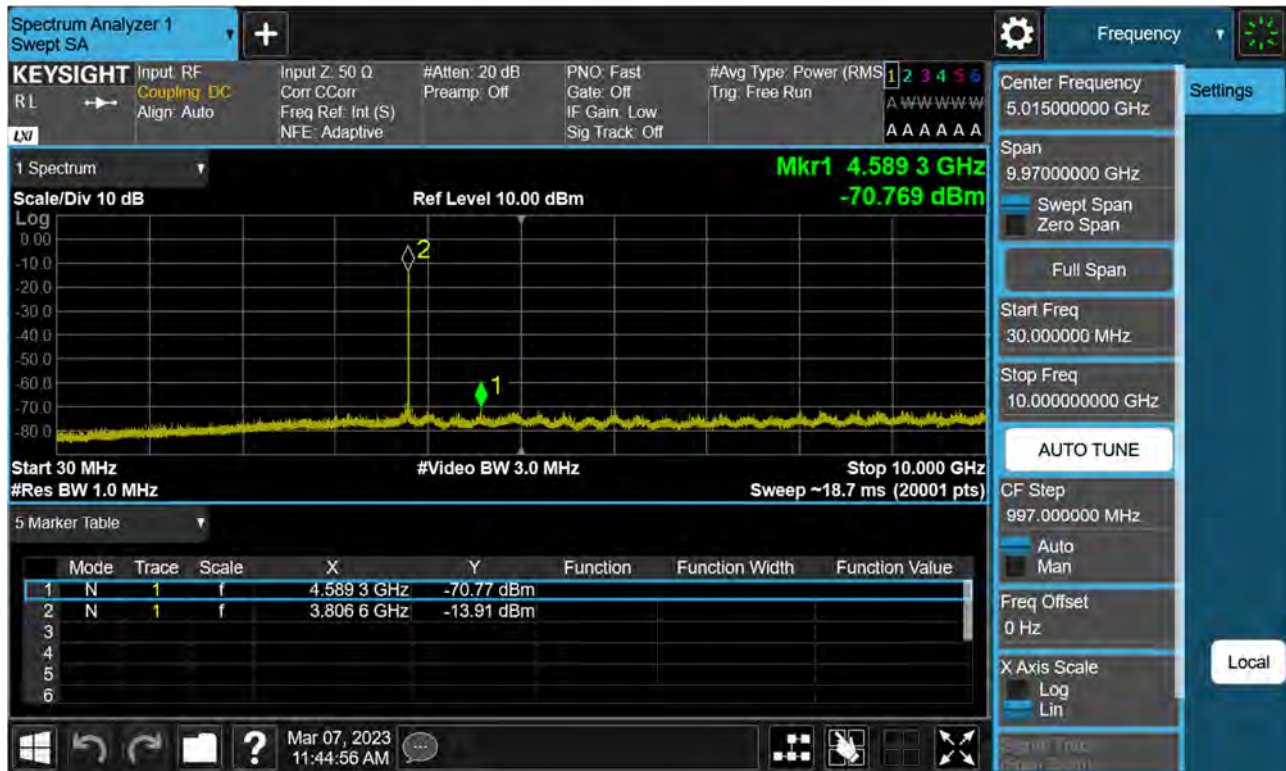
Sub6 n77(78). Conducted Spurious Plot_1 (656000ch_70 MHz_BPSK)
