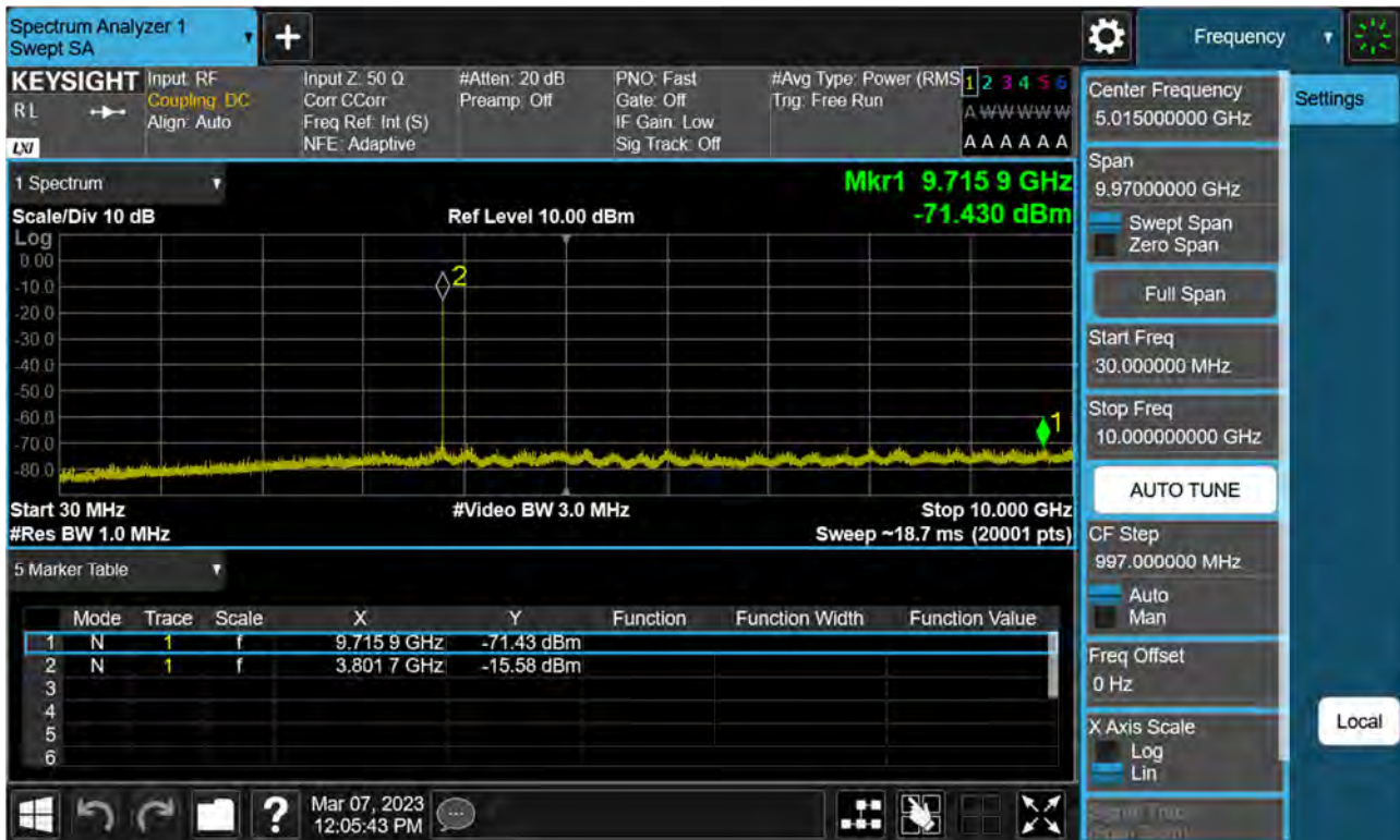
Sub6 n77(78). Conducted Spurious Plot_1 (656000ch_80 MHz_BPSK)
