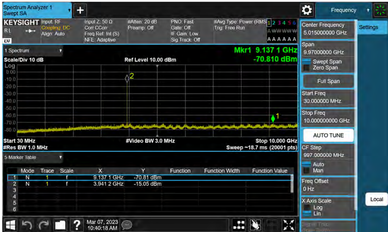
Sub6 n77(78). Conducted Spurious Plot_1 (664000ch_40 MHz_BPSK)
