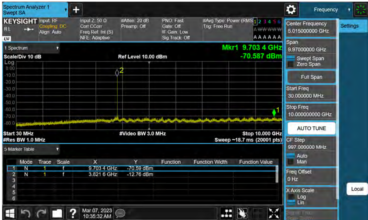
Sub6 n77(78). Conducted Spurious Plot_1 (656000ch_40 MHz_BPSK)
