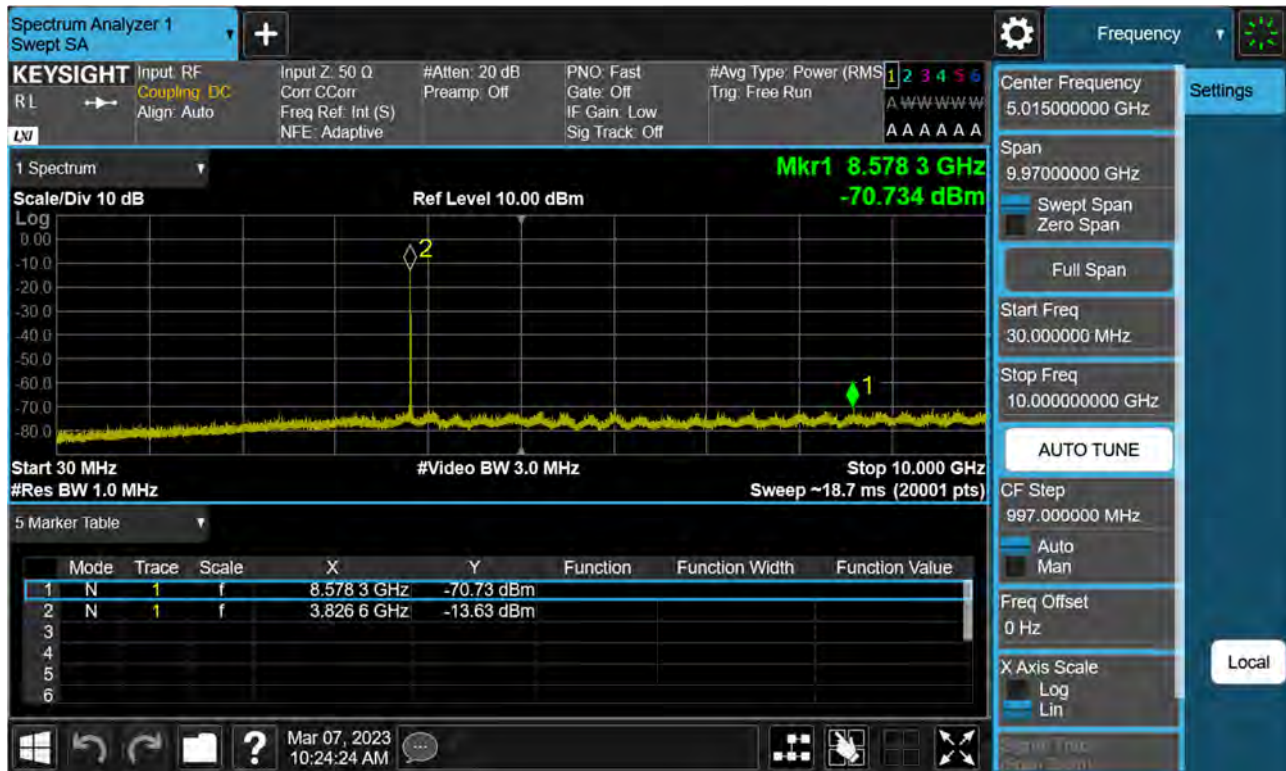
Sub6 n77(78). Conducted Spurious Plot_1 (656000ch_30 MHz_BPSK)
