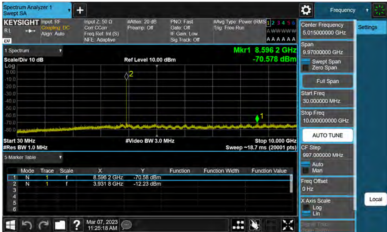
Sub6 n77(78). Conducted Spurious Plot_1 (663666ch_50 MHz_BPSK)
