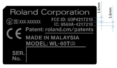
Withstands erosion of printing caused by friction. Material: Polycarbonate sheet Attached by permanent adhesive. The label will not come off during the product's lifetime.
