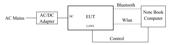
During the measurement of transmitter parameters, the EUT was continuously operating at maximum transmitting power and maximum data rate. The lowest, middle and highest channels were measured respectively.
