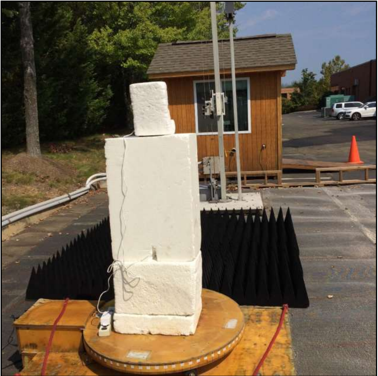
Photograph 2: Radiated Emissions Testing – Back View
