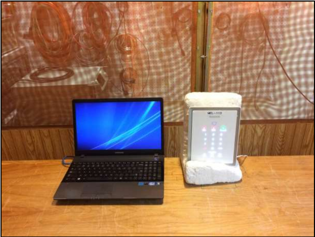
Photograph 3: AC Conducted Line Emissions Testing – Front View
