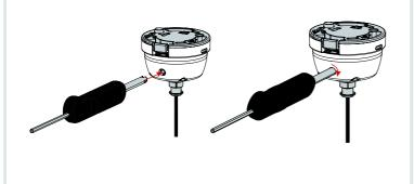
**2** Once the puck is loose, rotate the puck 45 degrees counterclockwise in relation to the tether. Lift the puck off of tether connection.
