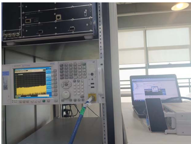
RF Conducted Test setup (BT/WIFI)
