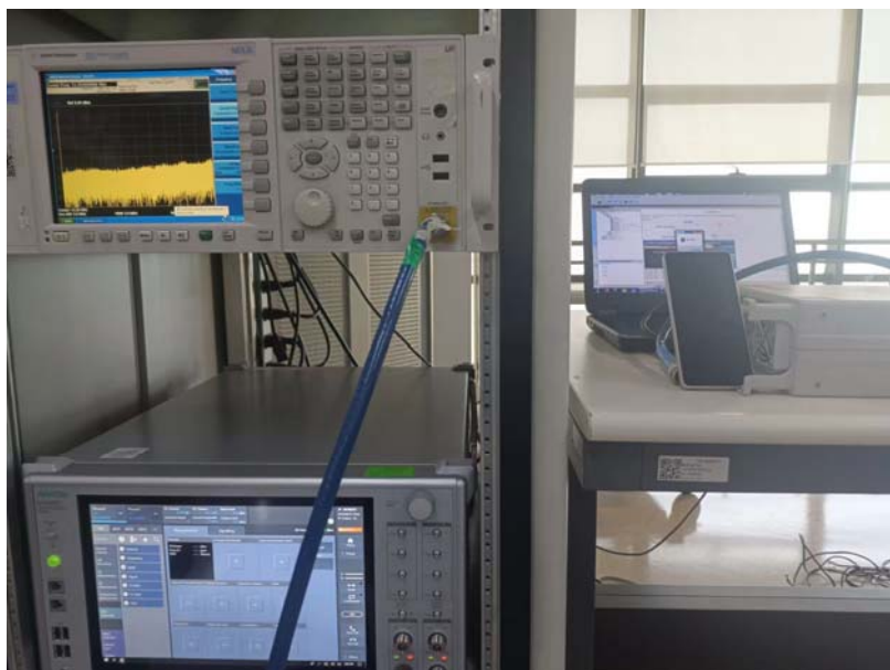
RF Conducted Test setup (GSM/WCDMA/LTE)
