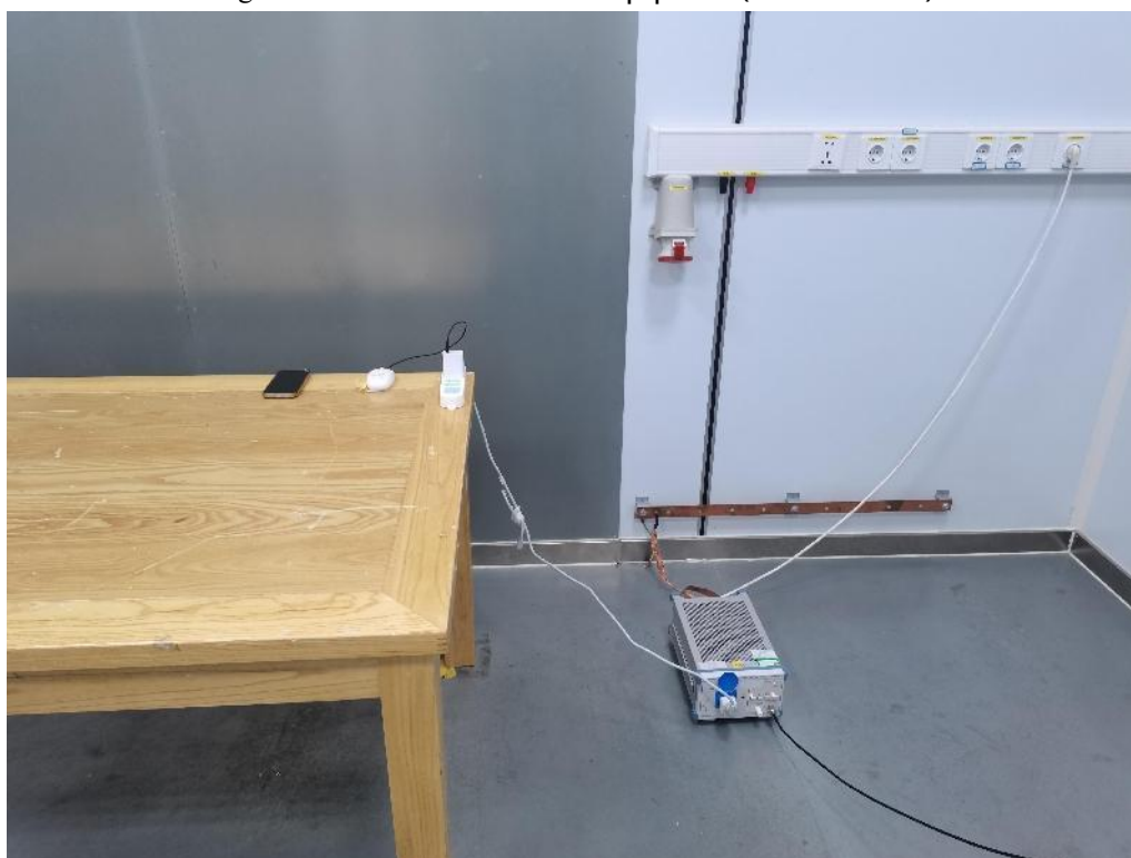
Fig. 4 Power line conducted emission setup photo
