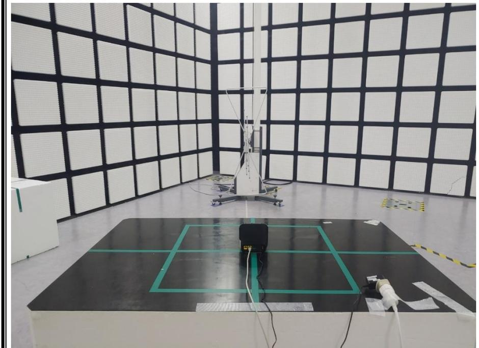
2) RADIATED RF MEASUREMENT SETUP (ABOVE 1 GHz)
