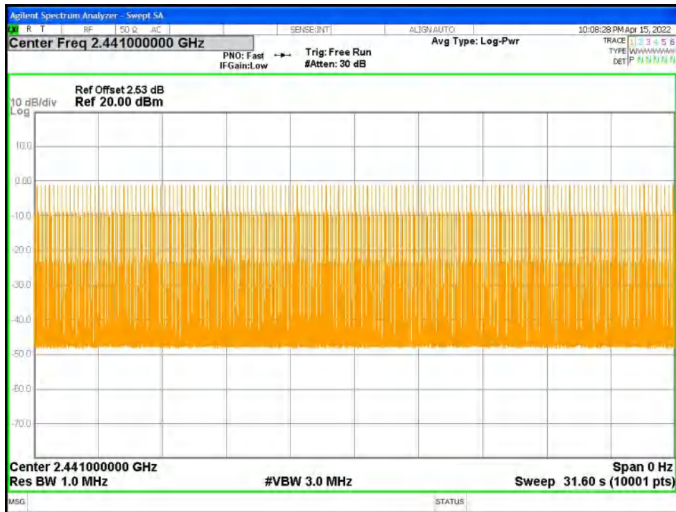
Dwell NVNT 1-DH5 2441MHz Ant1 One Burst
