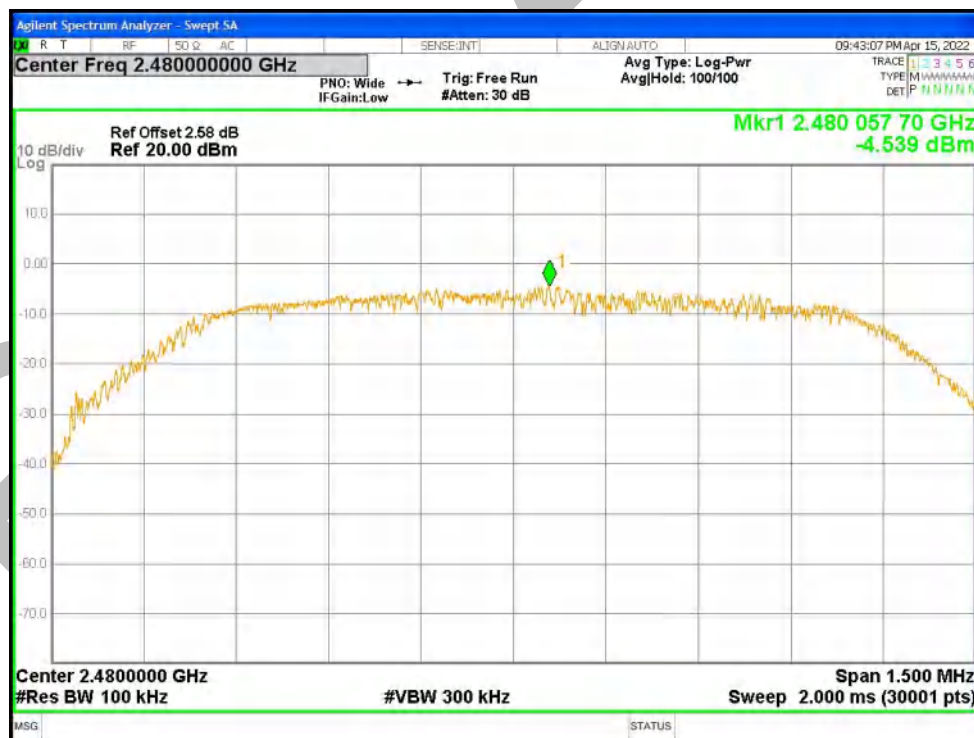
Tx. Spurious NVNT 2-DH1 2480MHz Ant1 Emission
