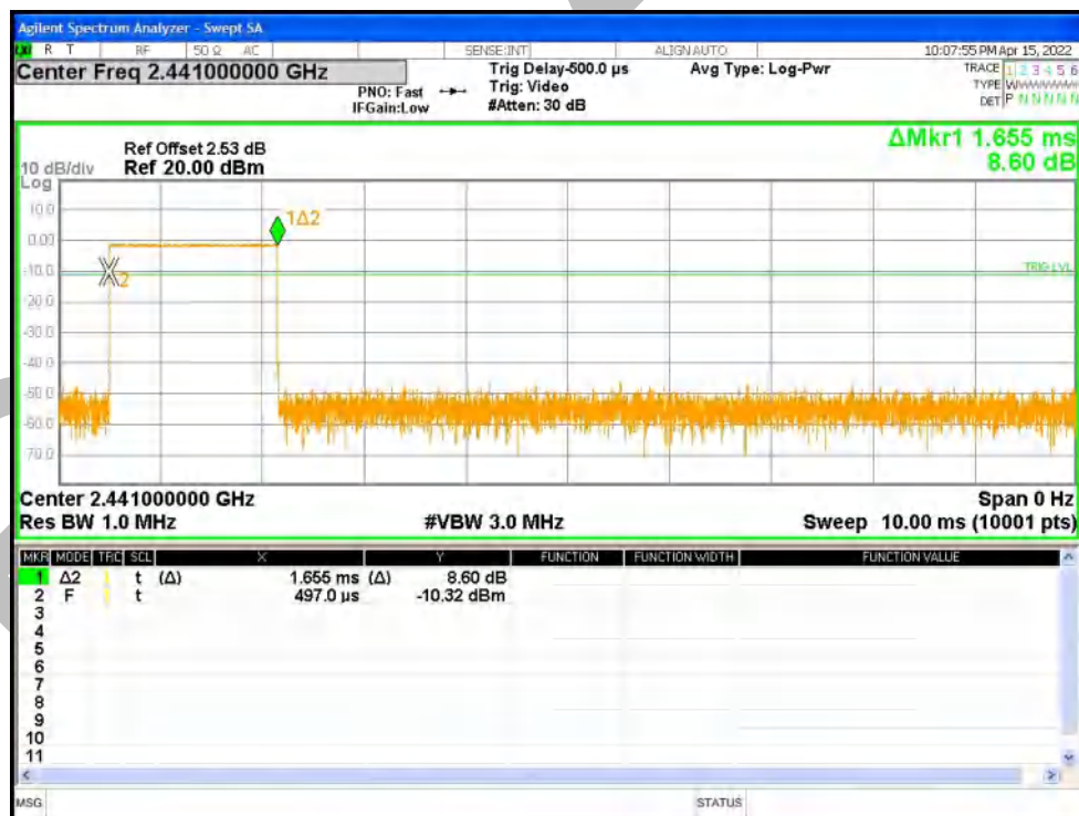
Dwell NVNT 1-DH3 2441MHz Ant1 Accumulated
