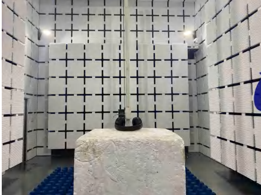
Radiated Spurious Emissions
