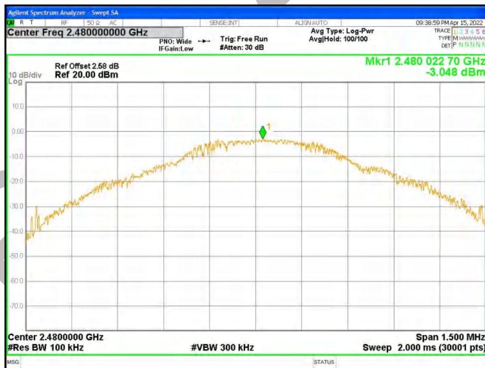
Tx. Spurious NVNT 1-DH1 2480MHz Ant1 Emission
