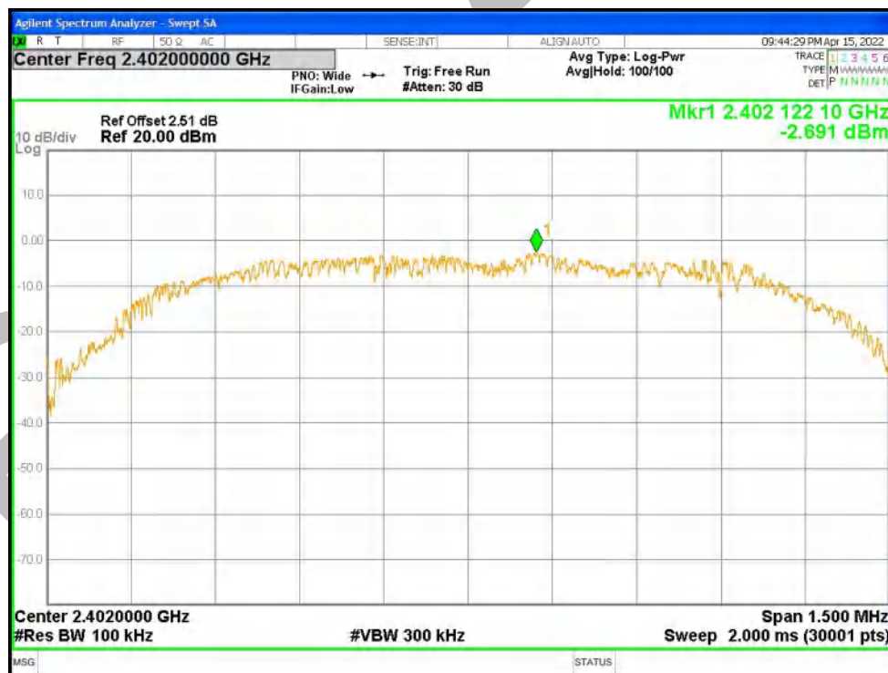
Tx. Spurious NVNT 3-DH1 2402MHz Ant1 Emission
