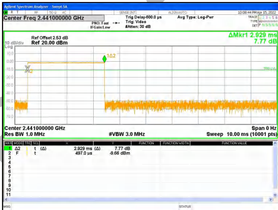
Dwell NVNT 1-DH5 2441MHz Ant1 Accumulated
