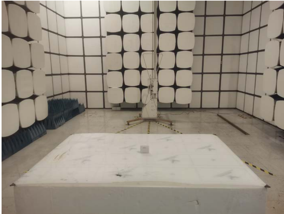
Spurious Emission Test Setup (Below 1GHz)
