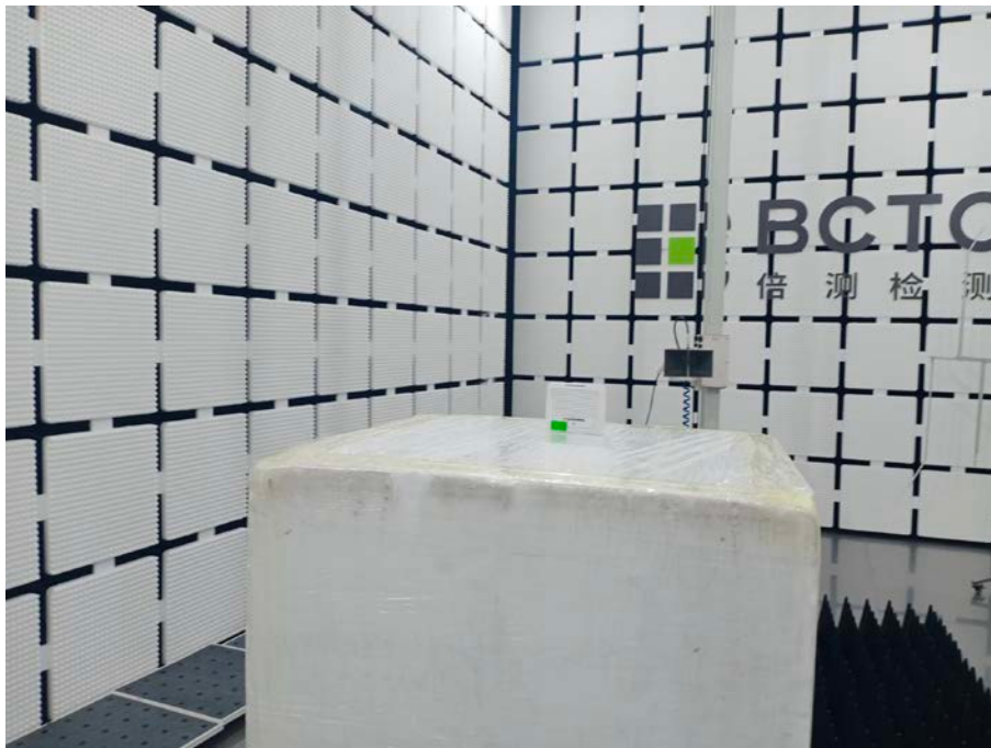
Spurious Emission Test Setup (Above 1GHz)
