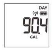
The screen shows the total water consumption each day starting at 0:00. The LCD displays the "DAY," and the unit is either L or GAL with a maximum display value of 9999999L or 999999GAL.
