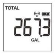
The LCD screen displays the total water consumption when the unit is powered on or starts operating. LCD displays the "TOTAL in either liter (L) or gallons (GAL)," and the total water consumption is updated every second.
