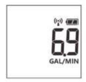
The screen displays the current flow rate value every second in units of L/Min or GAL/Min. The display does not show the leading zero; the maximum value indicated is 41.9L/Min or 11.0GAL/Min. If the flow rate exceeds this value, it will be displayed as HH.H L/Min or HH.H GAL/Min.
