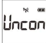
When the LCD is in the off state, press the button to show the current time and connection graph if the product is connected to the smartphone. If disconnected, it will show the disconnection graph. For a paired but disconnected device, it will display "-----." When the product is unpaired, it will show "Uncon." Pressing the button again will switch to mode 1.
