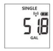
The LCD screen displays "SINGLE" water consumption in liters or gallons. Suppose the flow meter stops running for more than 30 seconds and restarts. In that case, it clears the original accumulated data, begins re-accumulating, and updates the display of real-time water consumption every second.
