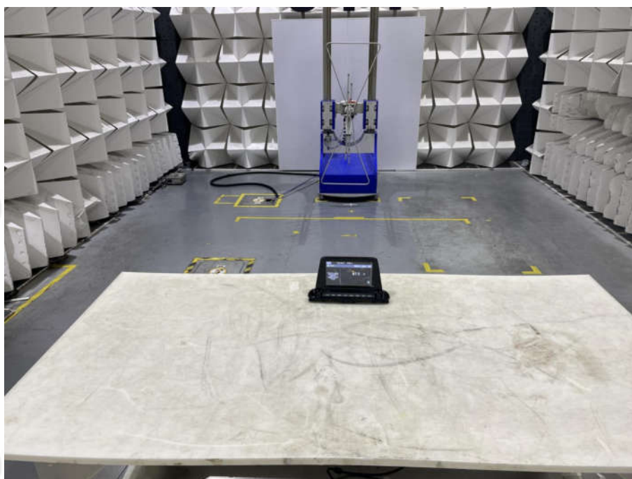
Radiated spurious emission Test Setup-1(Below 1GHz)
