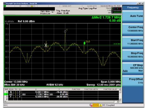
Note: The 20dB bandwidth was measured at all data rate and the worst case data was reported (This test item was tested at 424 kbps.)
