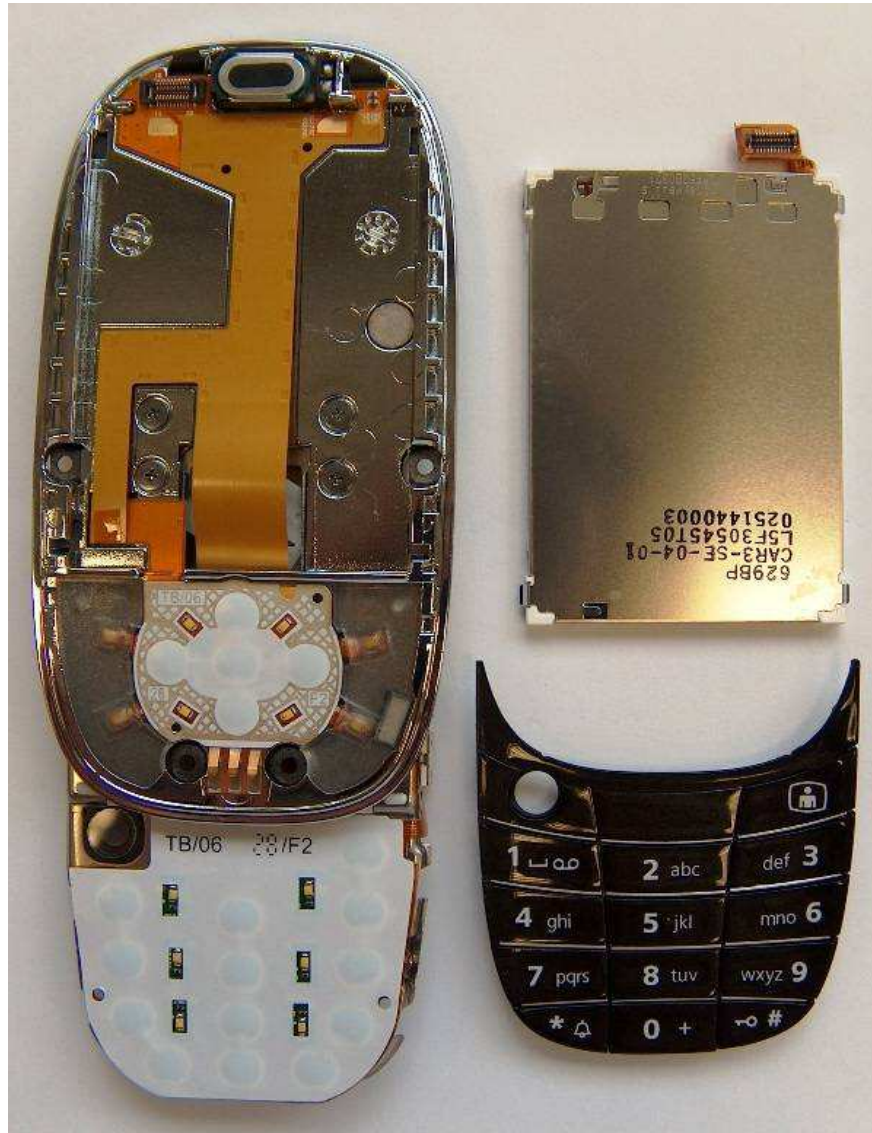
Disassemble Step 3: Display and Keypad separated from Slider
