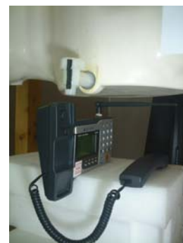
Figure 14.1 Body SAR Test Setup
