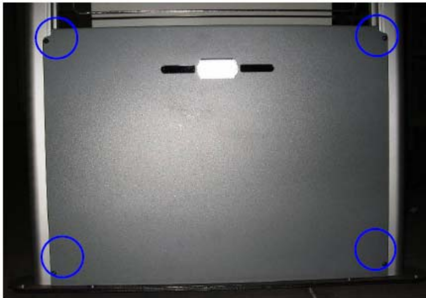
Figure 4.11: LSP3A Clear Bottom Plastic Cover (4 screws)
