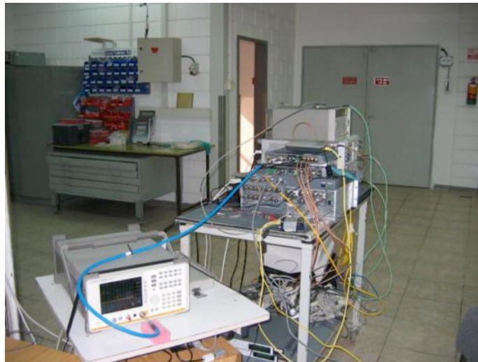
Photograph 1.7.1 Spurious emission test setup
