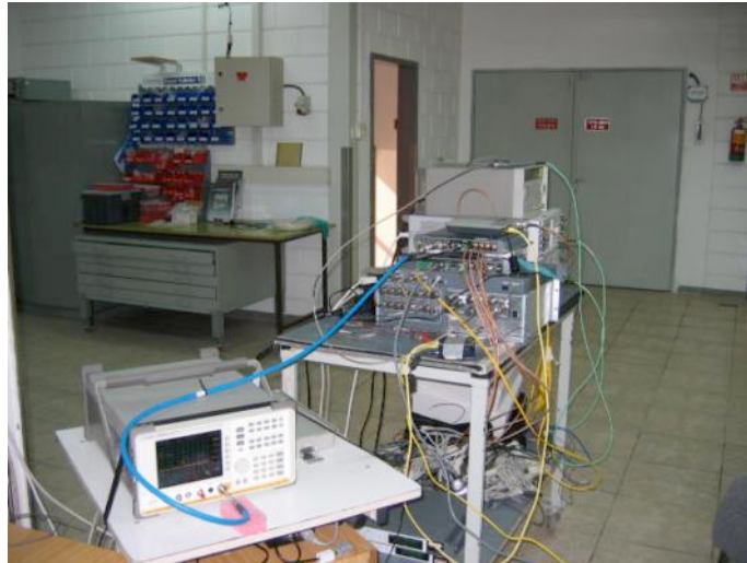
Photograph 1.6.1 Peak output power test setup
