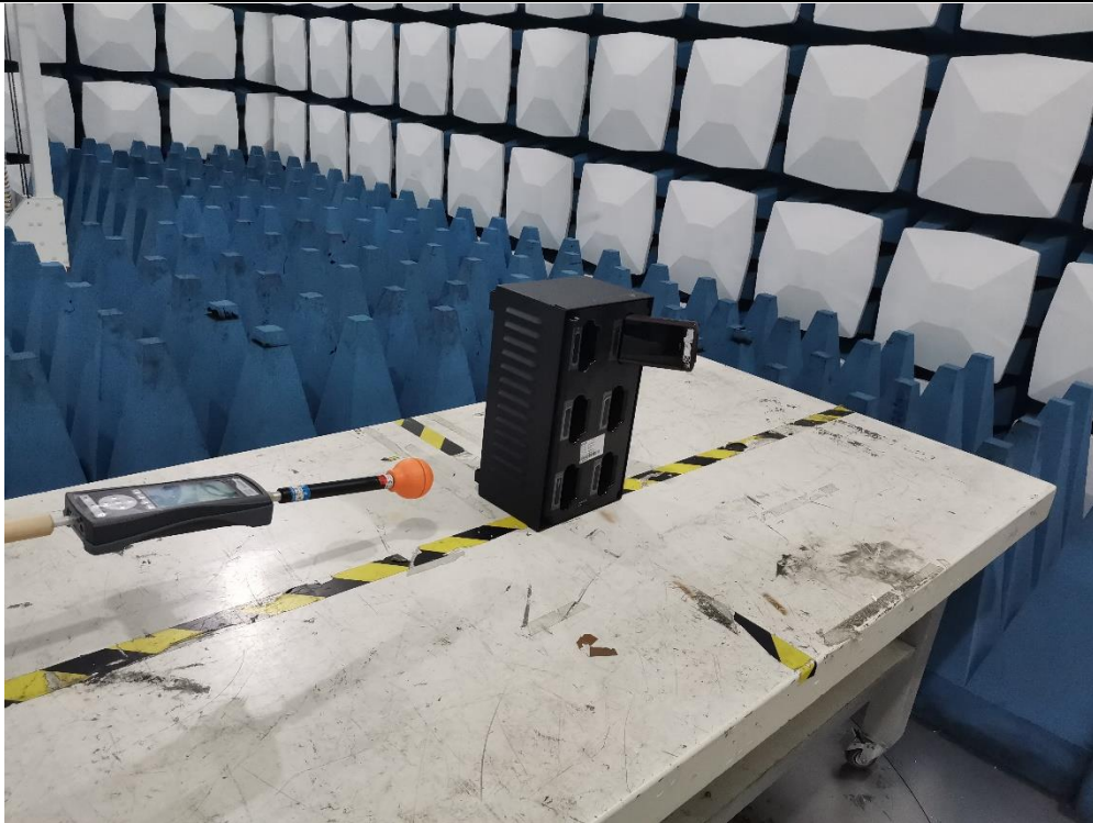
Description: RF Exposure Setup –Two devices Loaded 3kHz~100kHz
