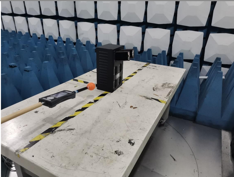
Description: RF Exposure Setup – Fully Loaded 3kHz~100kHz
