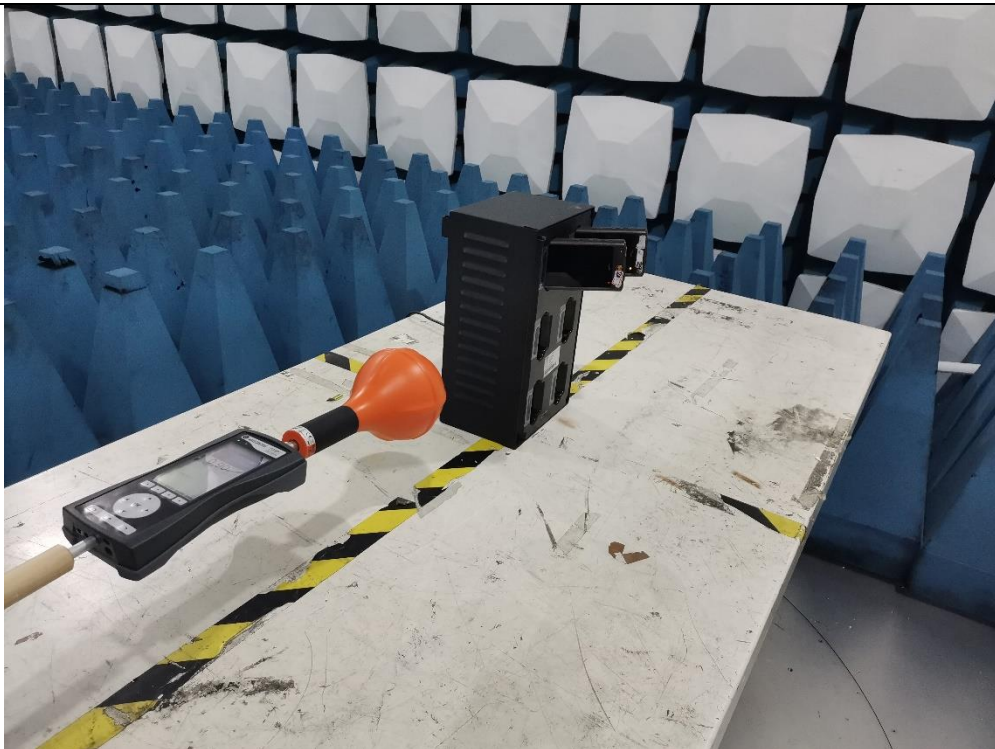
Description: RF Exposure Setup –Two devices Loaded 3kHz~100kHz
