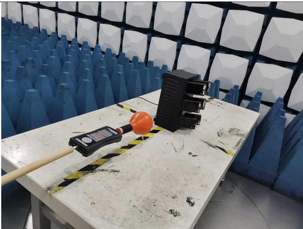
Description: RF Exposure Setup – Fully Loaded 3kHz~100kHz
