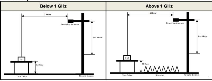
These measurements were performed at 3 test site. The equipment under test is placed on a non-conductive table 0.8 m or 1.5 m above a turntable which is flush with the ground plane and 3 meters from the receive antenna. For measurements above 1GHz absorbers are placed on the floor between the turn table and the antenna mast in such a way so as to maximize the reduction of reflections. For measurements below 1 GHz, the absorbers are removed.
