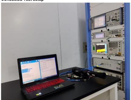
Conducted Emissions at AC Power Line (150kHz-30MHz)
