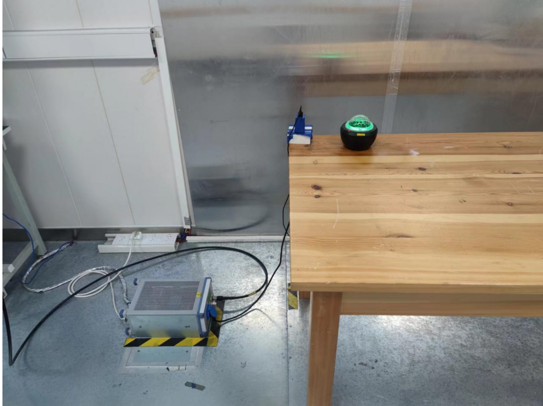
Conducted emission test setup
