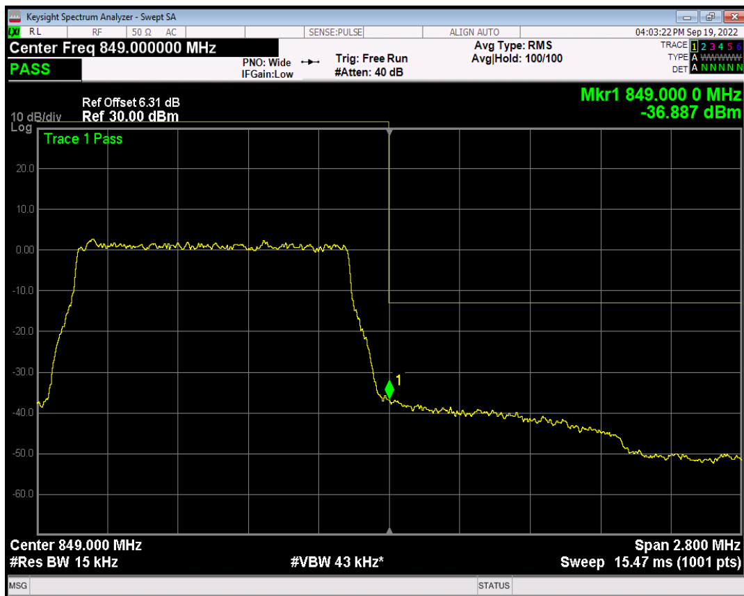
Band5 QAM16 BW=1.4MHz Channel=20643 RB Size=1 Position=#0
