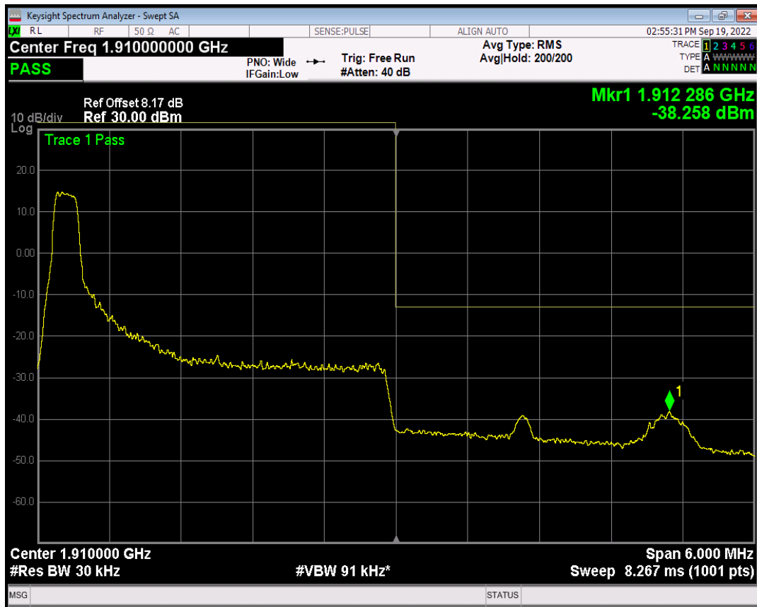
Band2 QAM16 BW=3MHz Channel=19185 RB Size=1 Position=#Max
