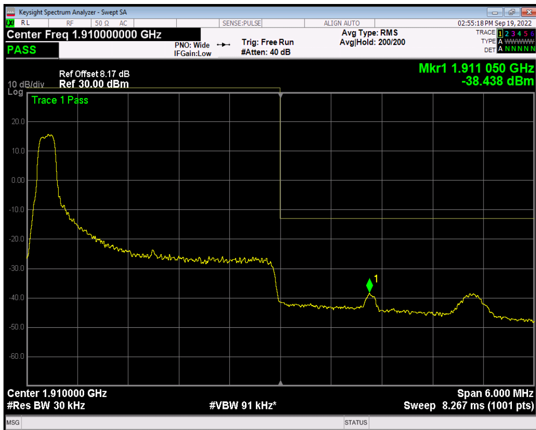
Band2 QPSK BW=3MHz Channel=19185 RB Size=1 Position=#Max
