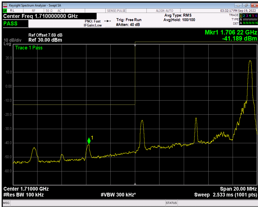
Band4 QPSK BW=10MHz Channel=20000 RB Size=50 Position=#0
