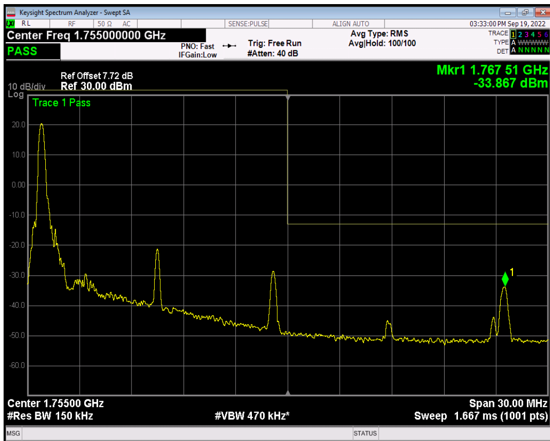
Band4 QPSK BW=15MHz Channel=20325 RB Size=1 Position=#Max
