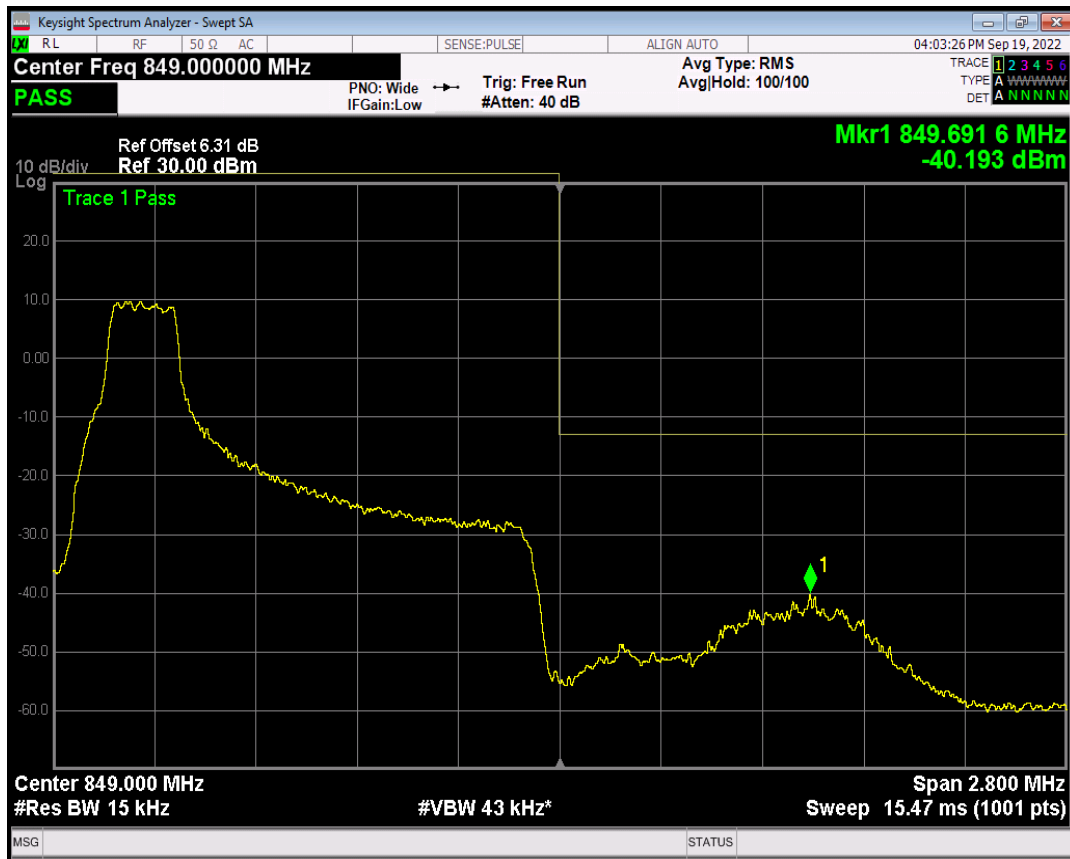
Band5 QAM16 BW=1.4MHz Channel=20643 RB Size=1 Position=#Max
