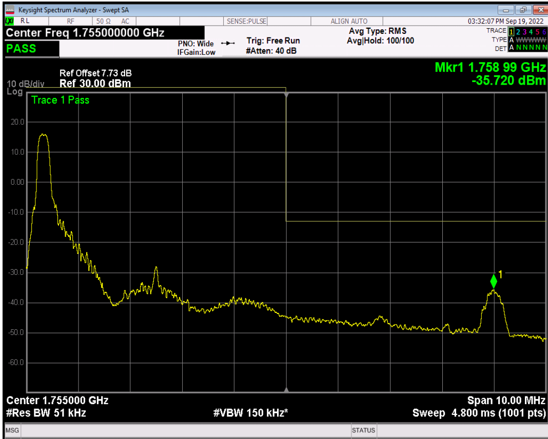
Band4 QAM16 BW=5MHz Channel=20375 RB Size=1 Position=#Max
