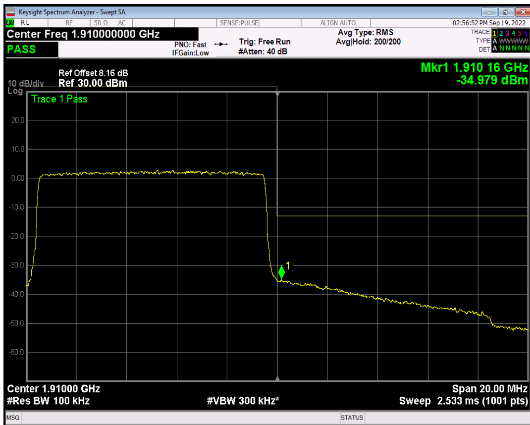
Band2 QAM16 BW=10MHz Channel=19150 RB Size=1 Position=#0
