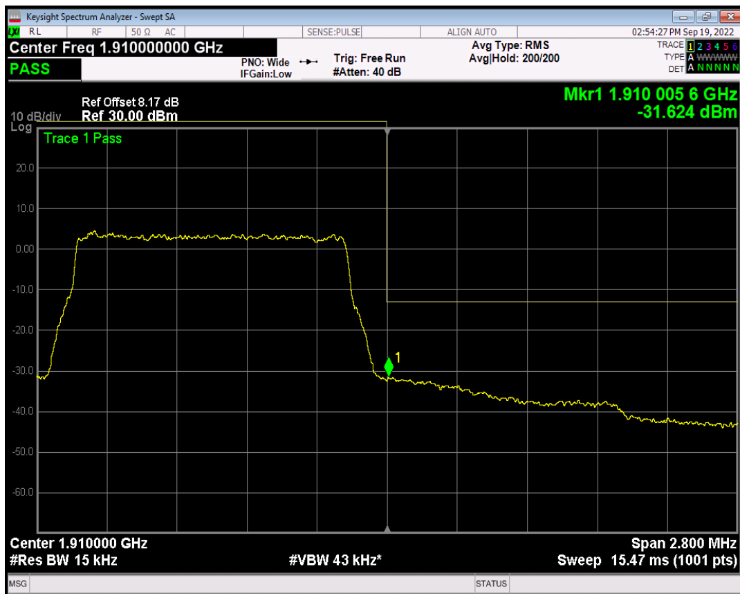
Band2 QAM16 BW=1.4MHz Channel=19193 RB Size=1 Position=#0
