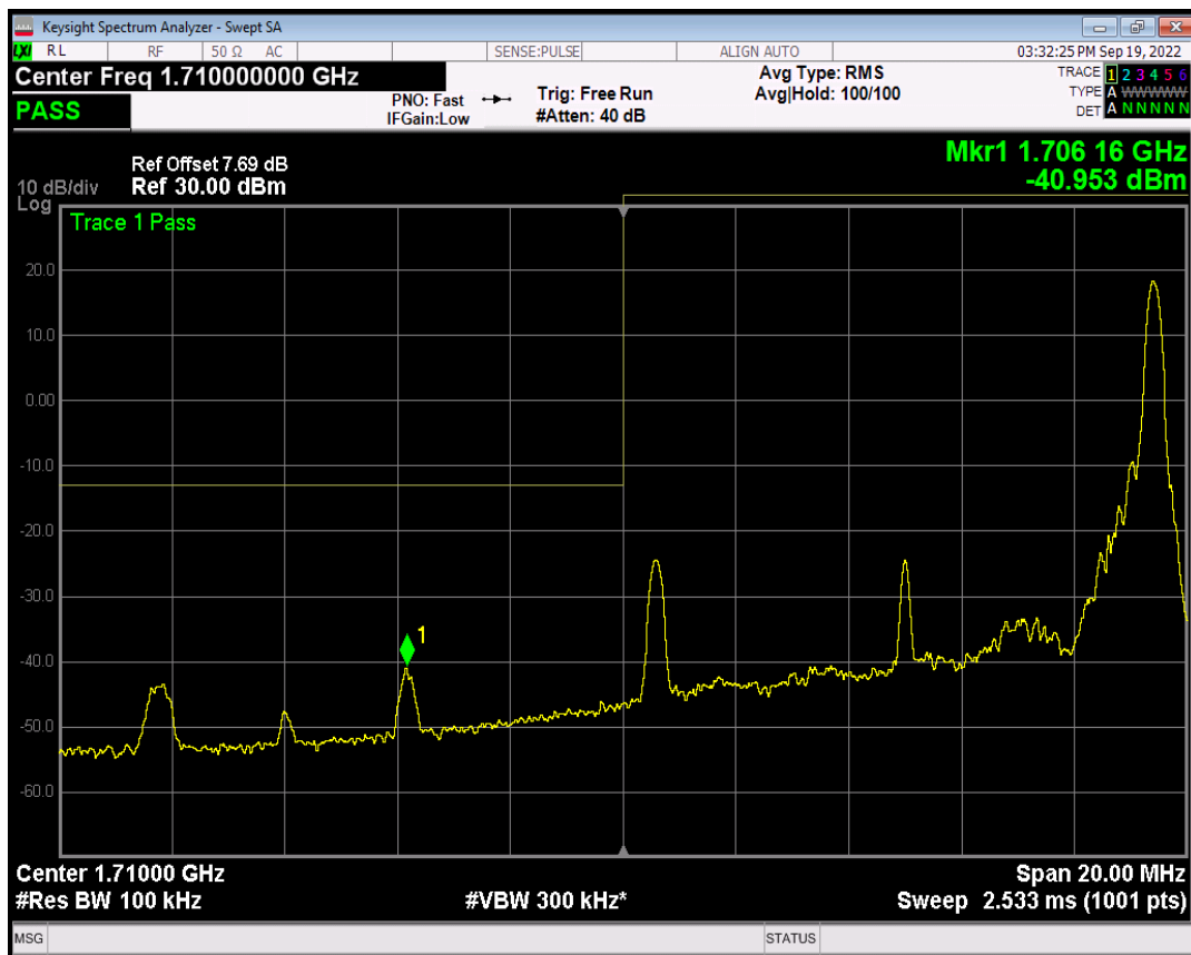
Band4 QAM16 BW=10MHz Channel=20000 RB Size=50 Position=#0
