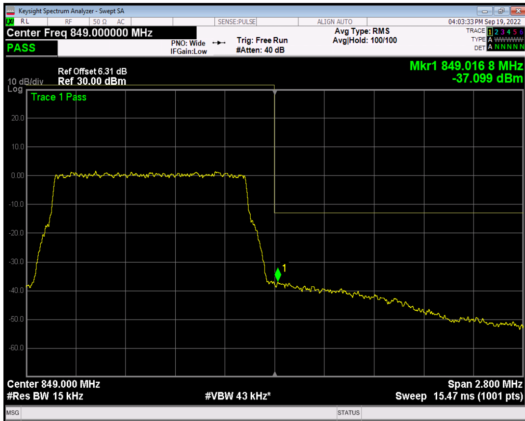
Band5 QPSK BW=3MHz Channel=20415 RB Size=1 Position=#0
