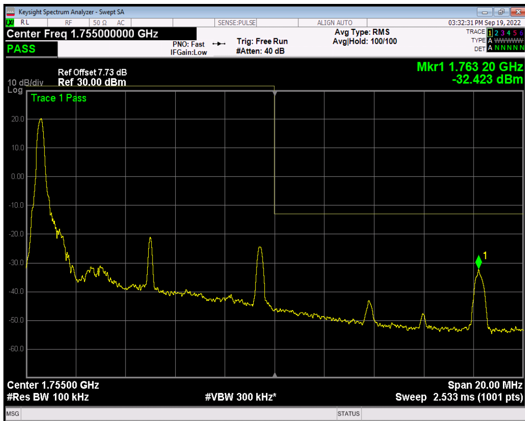
Band4 QPSK BW=10MHz Channel=20350 RB Size=1 Position=#Max
