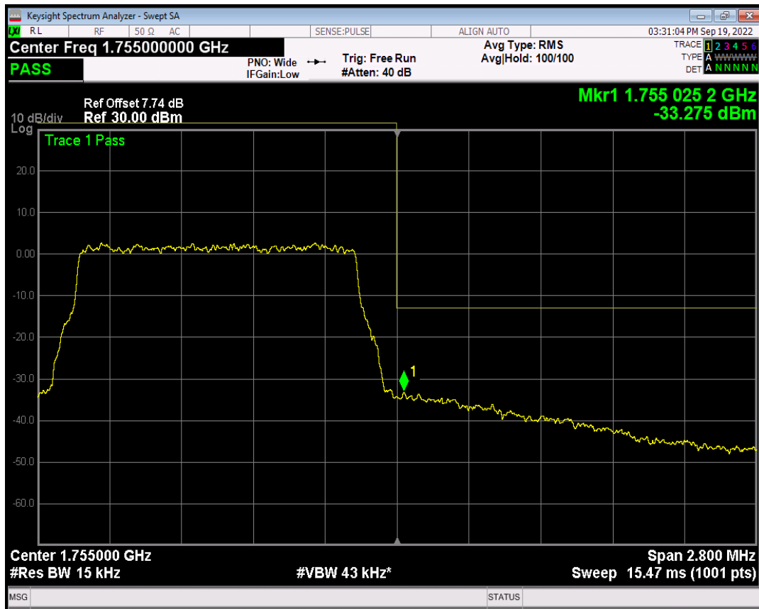
Band4 QPSK BW=3MHz Channel=19965 RB Size=1 Position=#0
