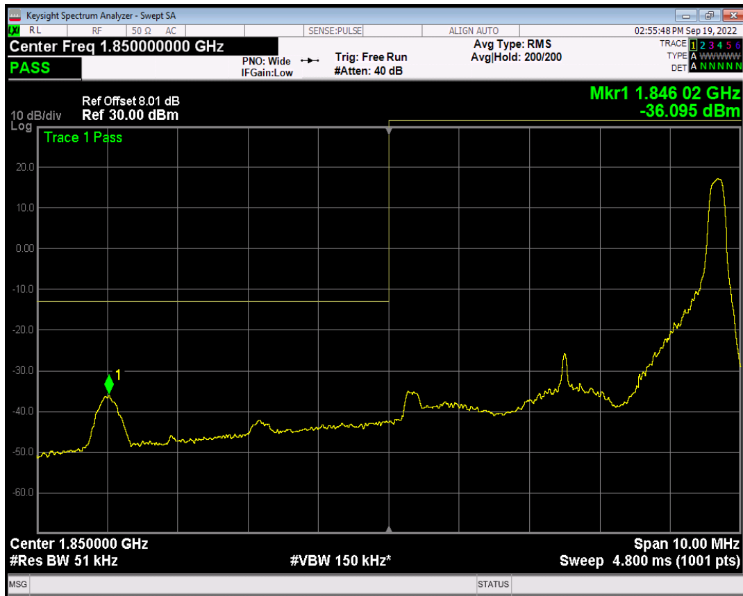
Band2 QPSK BW=5MHz Channel=18625 RB Size=25 Position=#0
