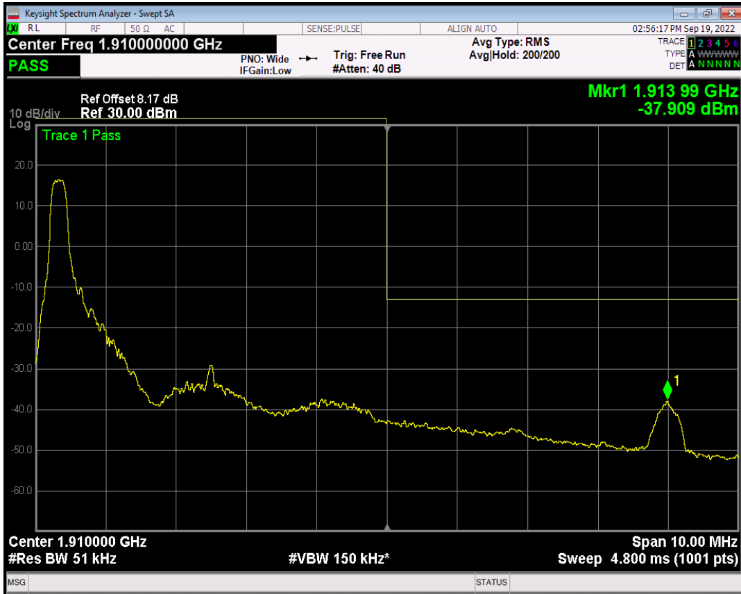
Band2 QAM16 BW=5MHz Channel=19175 RB Size=1 Position=#Max
