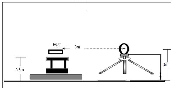
(B) Radiated Emission Test-Up Frequency 30MHz~1GHz
