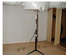
Figure 9.1 Dipole Verification Test Setup Diagram & Photo
