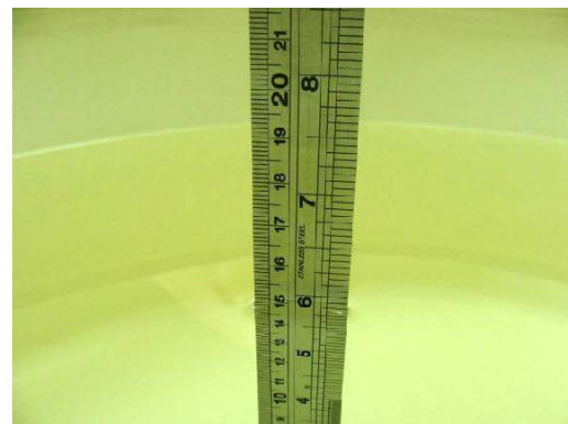
Fig 7.2 Photo of Liquid Height for Body SAR
