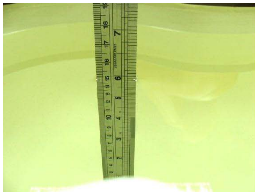
Fig 7.1 Photo of Liquid Height for Head SAR
