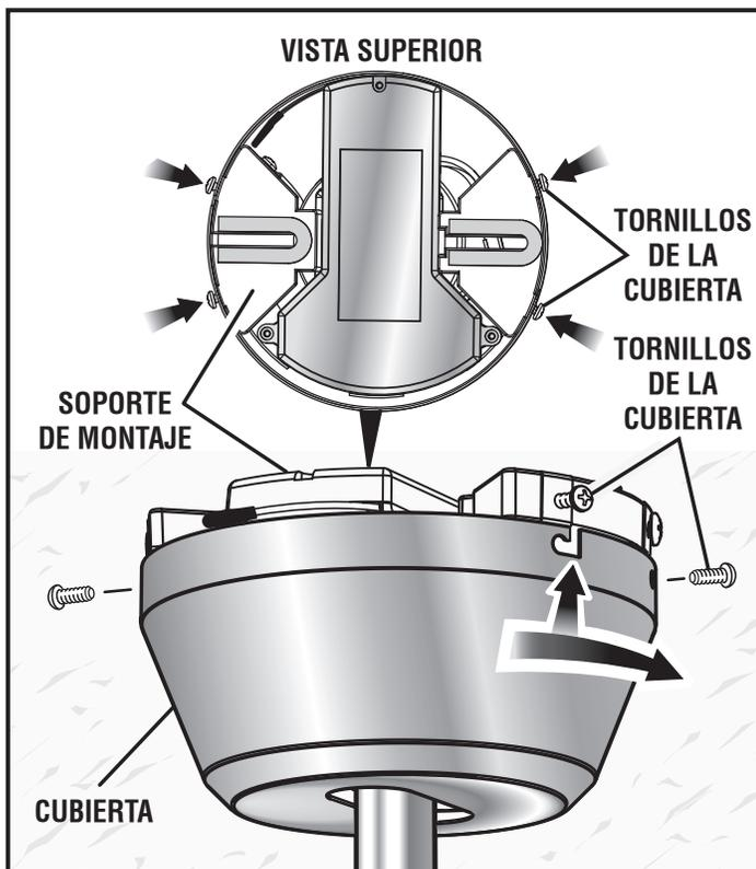
**NOTE:** If the canopy won't align with the screw holes, you may have overtightened the ceiling mounting bracket screws when securing the bracket to the outlet box. Remove the ceiling fan and loosen the screws just enough to allow the outlet box to become flush with the sheetrock, but not so much that the ceiling fan bracket is no longer securely fastened to the outlet box.
