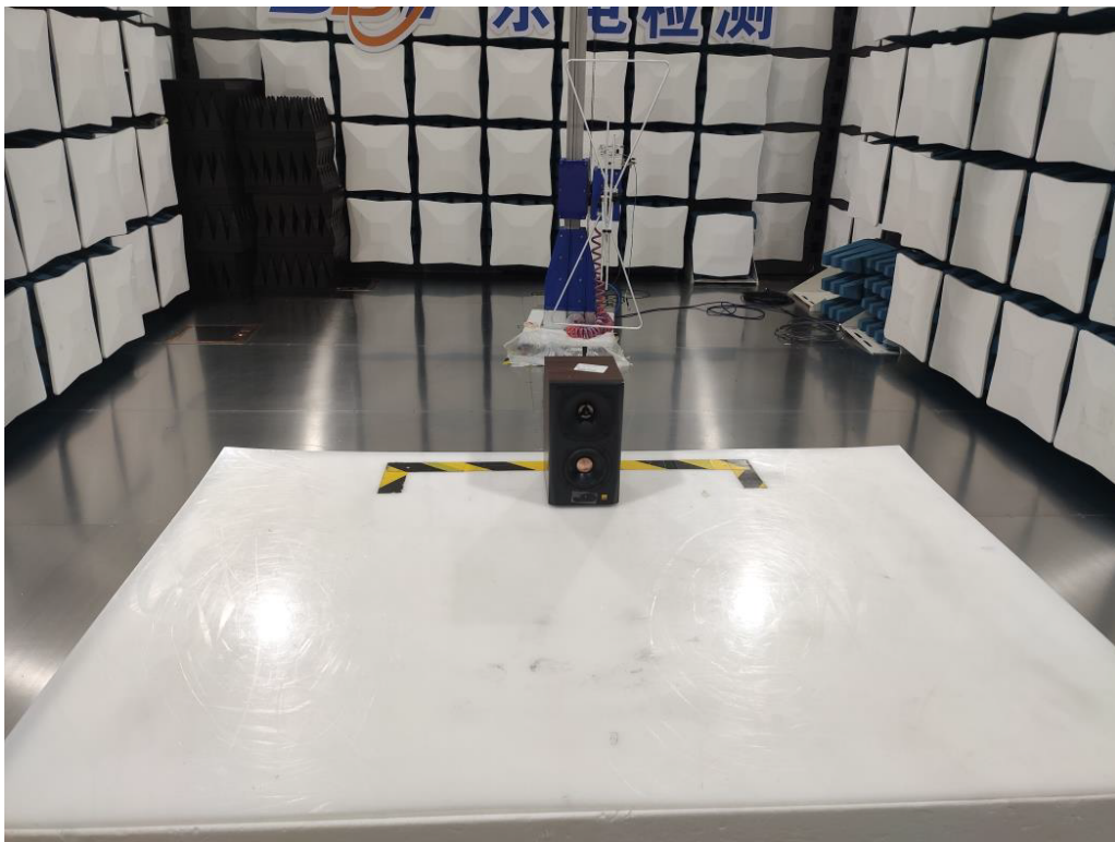
Photograph 2: Set-up for Radiated Spurious Emission, below 1GHz
