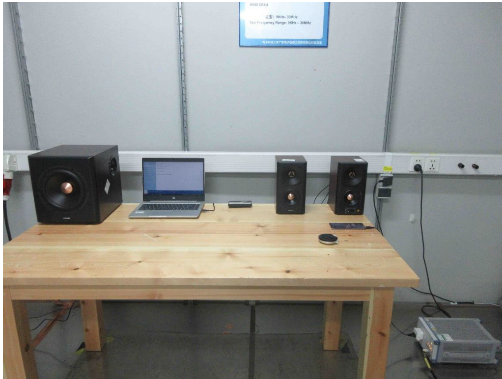
Photograph 1: Set-up for Conducted Emission on AC Mains
