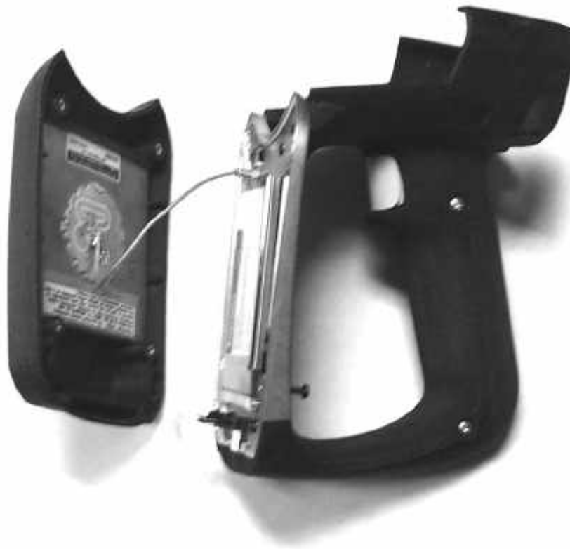
View of Interior of IP3 showing 915 PC Card-6
