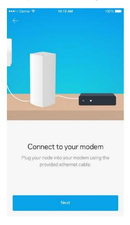
If you have more than one node, they can be set up anywhere within range of another working node. Only one node has to be wired to the modem or modem router. Don't worry, the app will help you place your nodes.
