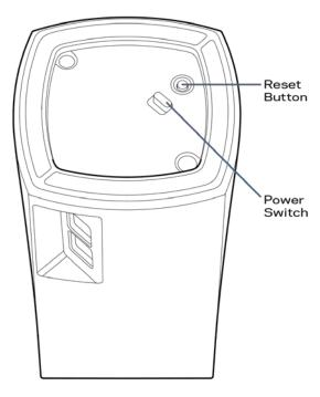
Reset button—Press and hold until the light on top of the node turns red, fades and flashes bright red again to reset the node to its factory defaults.
