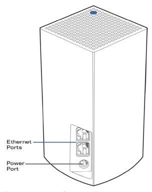
Ethernet ports—Connect Ethernet cables to these Gigabit Ethernet (10/100/1000) ports and to other wired devices on your network. If you have more than one node in your Velop system, use one of these ports to connect to your modem or modem router.
