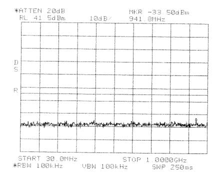
Intermodulation Close Lower GSM PCS 1900 MHz EFC Band
