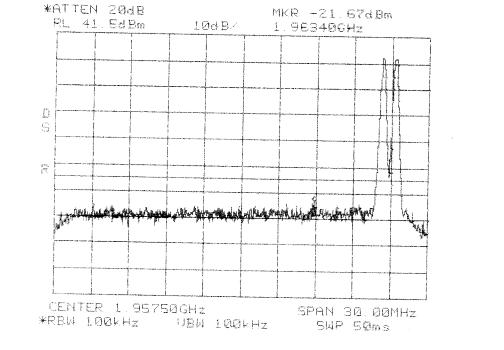
Intermodulation Close Upper GSM PCS 1900 MHz DBE Band
