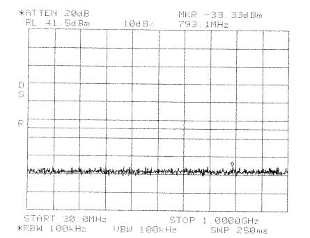
Intermodulation Close Lower TDMA PCS 1900 MHz EFC Band
