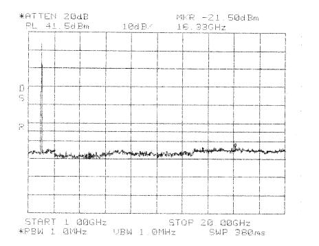
Intermodulation Close Upper GSM PCS 1900 MHz DBE Band
