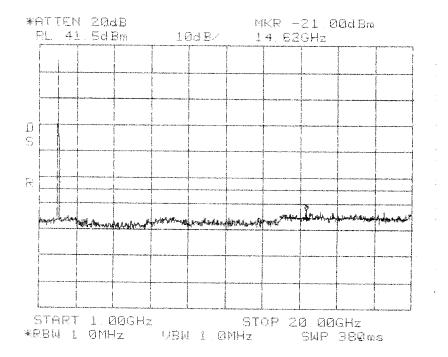
Intermodulation Close Upper TDMA PCS 1900 MHz DBE Band
