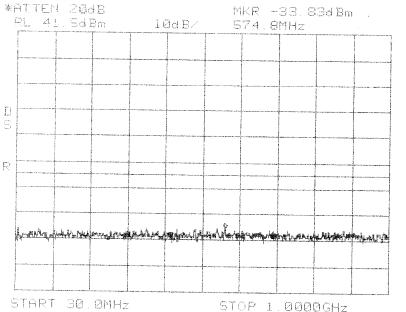
STHRT BULUMHZ STOP 1.0000GHz \*RBW 100kHz - VBW 100kHz - SWP 250ms Intermodulation Close Lower TDMA PCS 1900 MHz DBE Band
