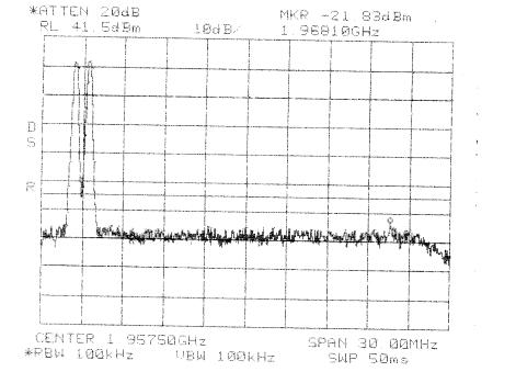
Intermodulation Close Lower GSM PCS 1900 MHz DBE Band
