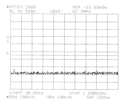
Intermodulation Close Upper GSM PCS 1900 MHz EFC Band
