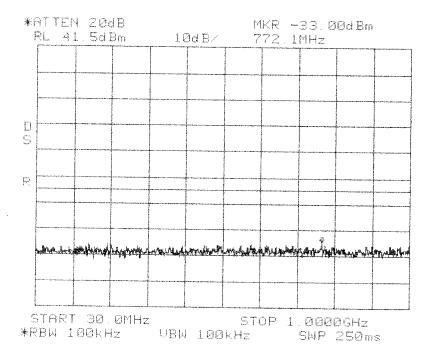
Intermodulation Close Lower GSM PCS 1900 MHz BEF Band
