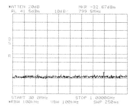
Intermodulation Close Upper GSM PCS 1900 MHz BEF Band
