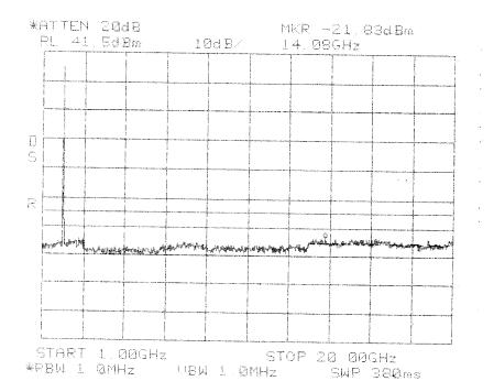
Intermodulation Close Lower TDMA PCS 1900 MHz DBE Band
