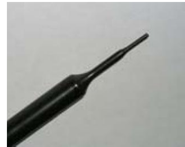
Picture C.2 Near-field Probe
