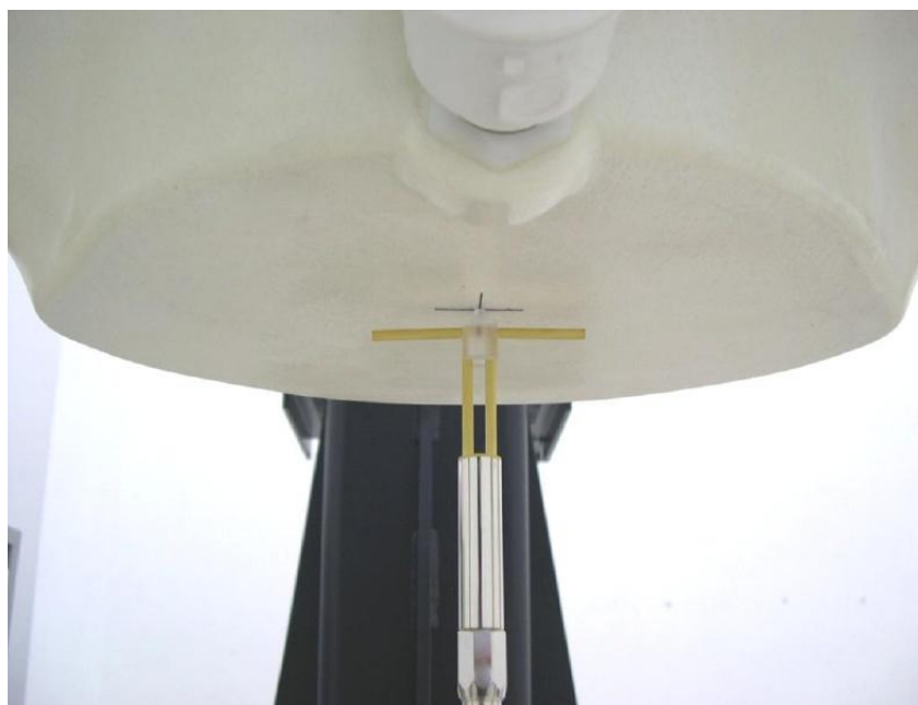
Picture 8.2 Photo of Dipole Setup
