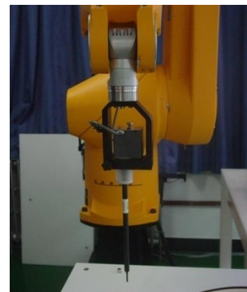
Picture C.3 E-field Probe
