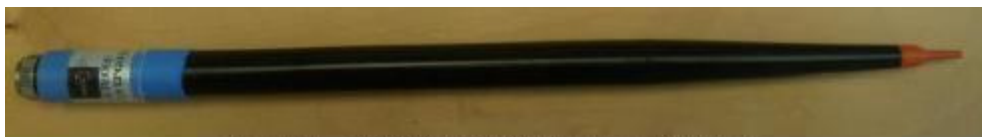
Figure 1 – MVG COMOSAR Dosimetric E-field Dipole
