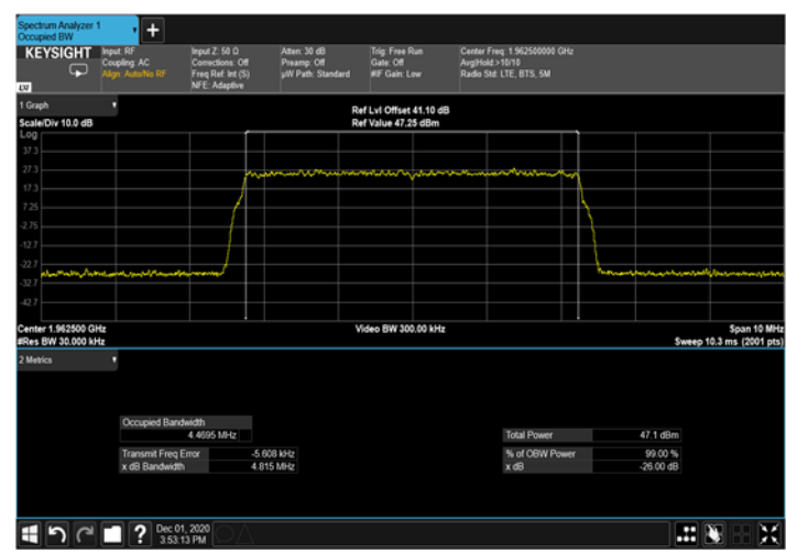
Figure 357: 16QAM 5MHz B.W.; 1962.5MHz Output – 4G
