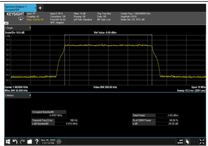
Figure 345: QPSK 5MHz B.W.; 1962.5MHz Input – 4G
