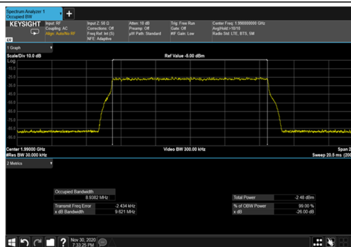
Figure 331: 16QAM 10MHz B.W.; 1990MHz Input – 4G
