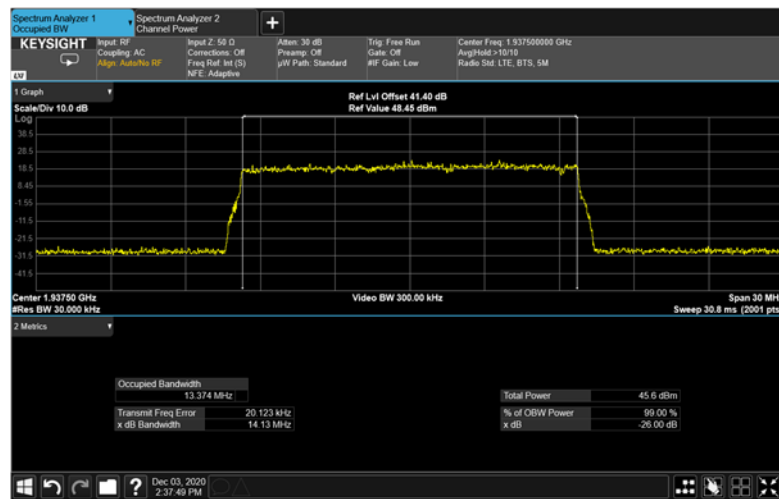
Figure 362: 16QAM 15MHz B.W.; 1937.5MHz Output – 4G
