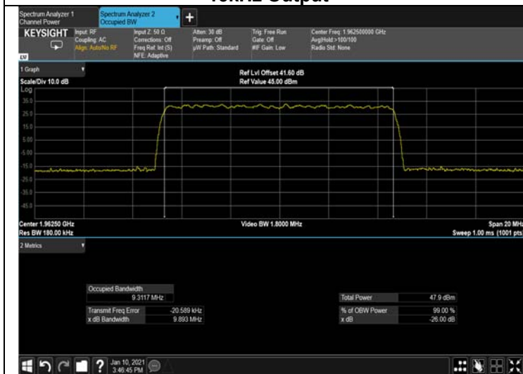
Figure 295: 256QAM 10MHz B.W.; 1962.5MHz, 15kHz Output
