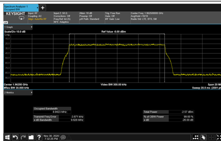
Figure 330: 16QAM 10MHz B.W.; 1962.5MHz Input – 4G
