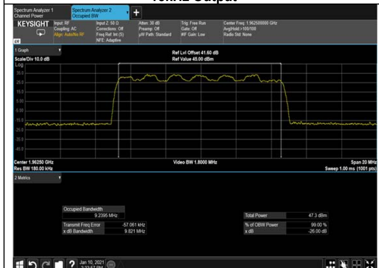
Figure 259: 16QAM 10MHz B.W.; 1962.5MHz, 15kHz Output
