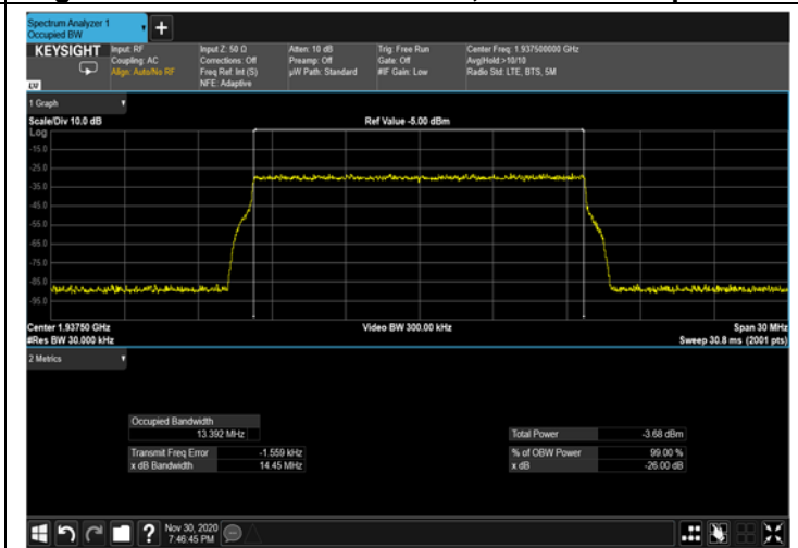
Figure 341: 64QAM 15MHz B.W.; 1937.5MHz Input – 4G
