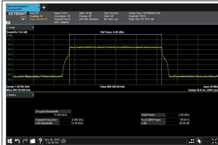
Figure 350: QPSK 15MHz B.W.; 1937.5MHz Input – 4G
