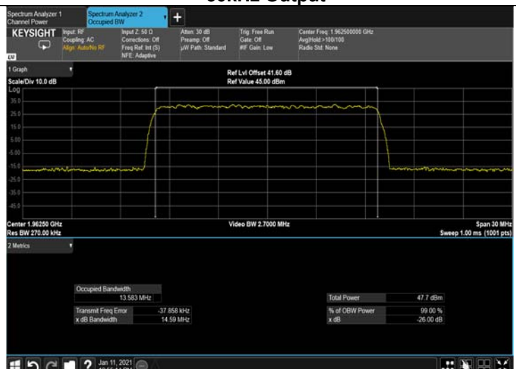
Figure 302: 256QAM 15MHz B.W.; 1962.5MHz, 30kHz Output
