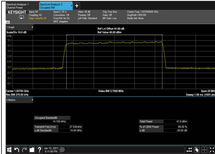
Figure 299: 256QAM 15MHz B.W.; 1937.5MHz, 15kHz Output
