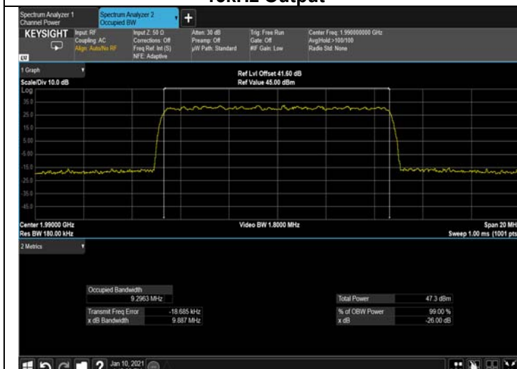
Figure 297: 256QAM 10MHz B.W.; 1990.0MHz, 15kHz Output
