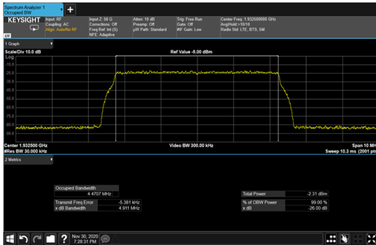
Figure 326: 16QAM 5MHz B.W.; 1932.5MHz Input – 4G
