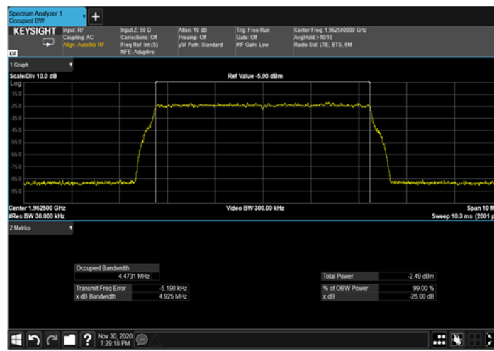
Figure 327: 16QAM 5MHz B.W.; 1962.5MHz Input – 4G
