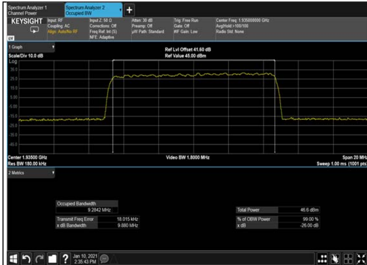
Figure 293: 256QAM 10MHz B.W.; 1935.0MHz, 15kHz Output
