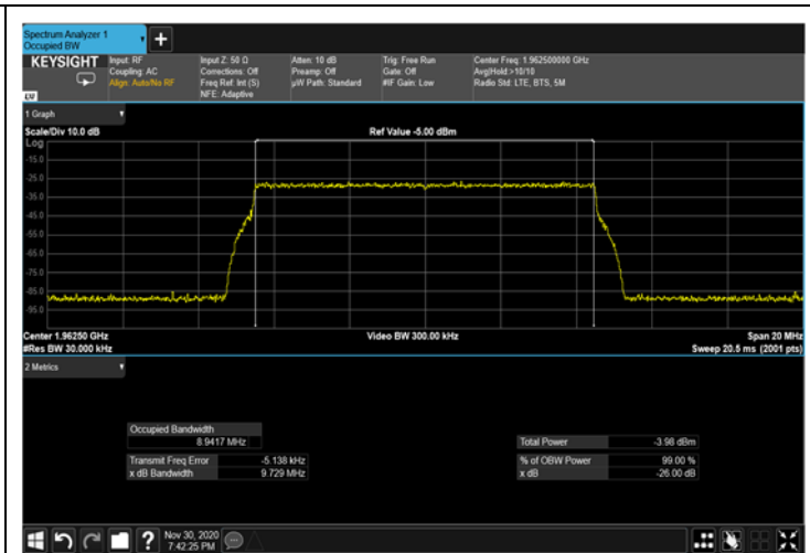
Figure 339: 64QAM 10MHz B.W.; 1962.5MHz Input – 4G
