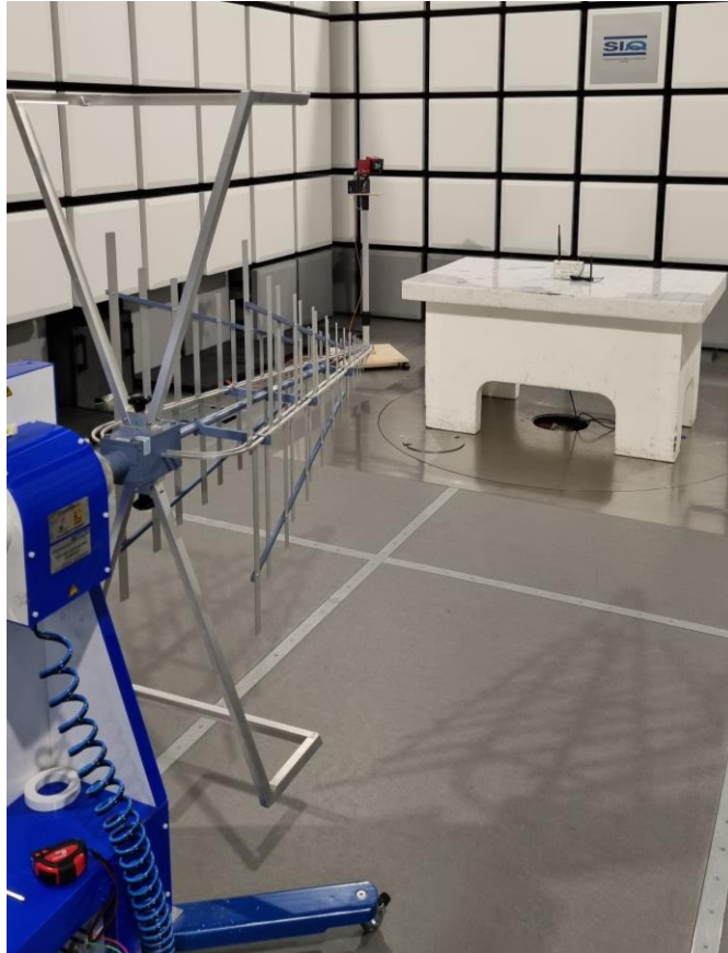
Figure 3: Spurious emission 30 MHz-1000 MHz
