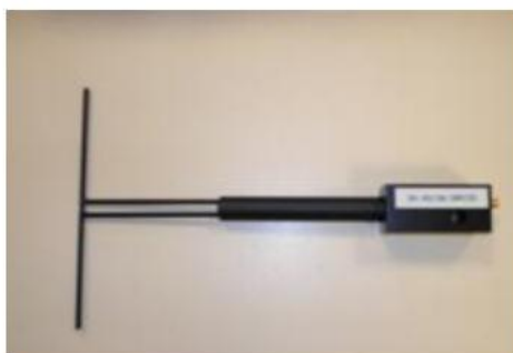
Figure 1 – Satimo COMOSAR Validation Dipole
