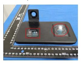
① Wireless charging area for mobile phone which include one coil.
