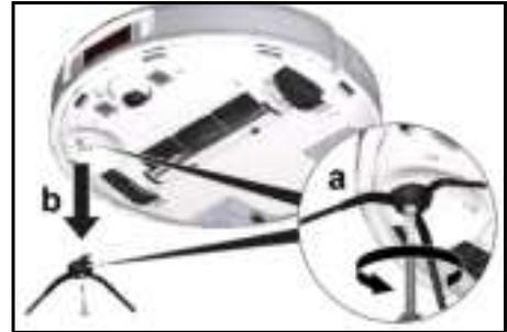
3. Tighten new side brush with a Phillips screwdriver.
