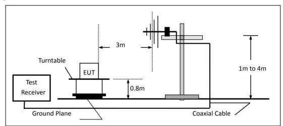
(c) For radiated emissions above 1000MHz
