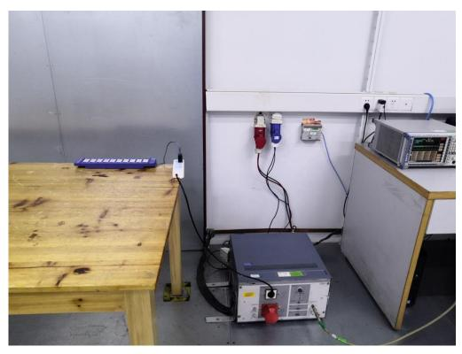
RADIATED EMISSION TEST SETUP BELOW 30MHz
