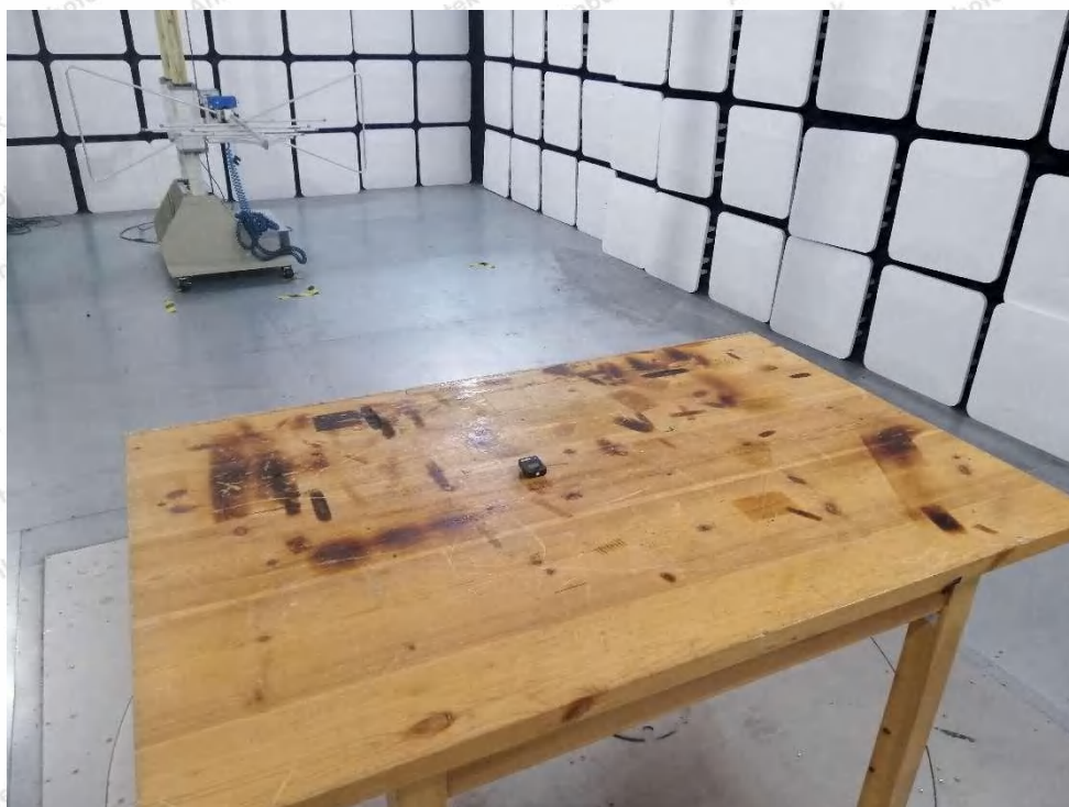
Photo of Radiation Emission Test
