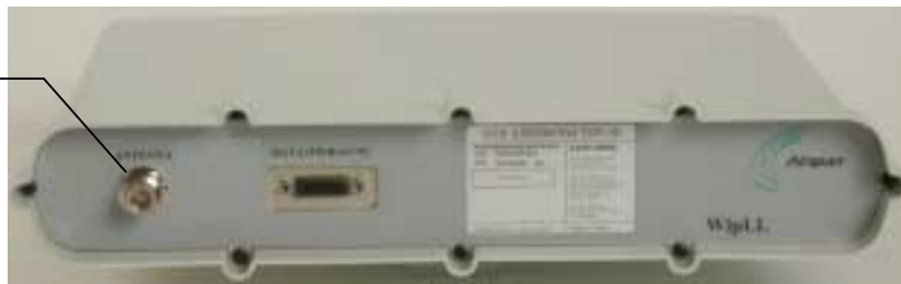
Figure 4-9: BSR model with N-type antenna connector
