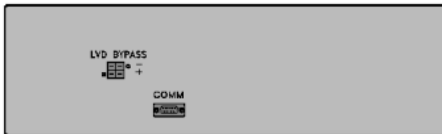
Figure 7-10: DC Distribution Rack rear view
