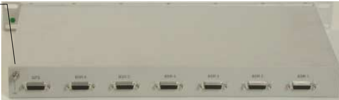
Figure 5-11: BSDU rear panel with grounding lug screw
